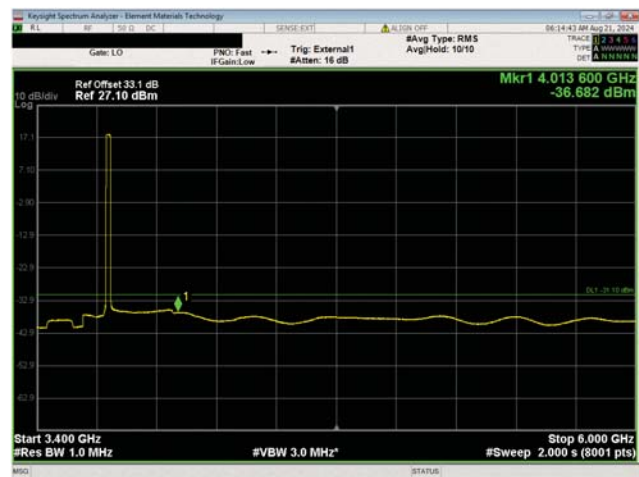
Port 1 20 MHz Channel Bandwidth QPSK Modulation Mid Channel, 3840.00 MHz
