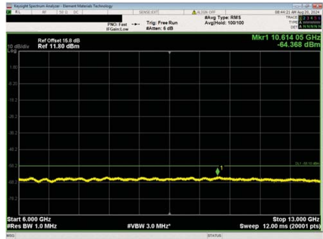
Port 1 40 MHz Channel Bandwidth QPSK Modulation Mid Channel, 3500.01 MHz
