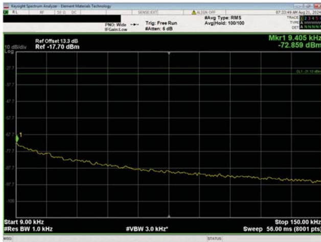
Port 1 100 MHz Channel Bandwidth QPSK Modulation Mid Channel, 3840.00 MHz
