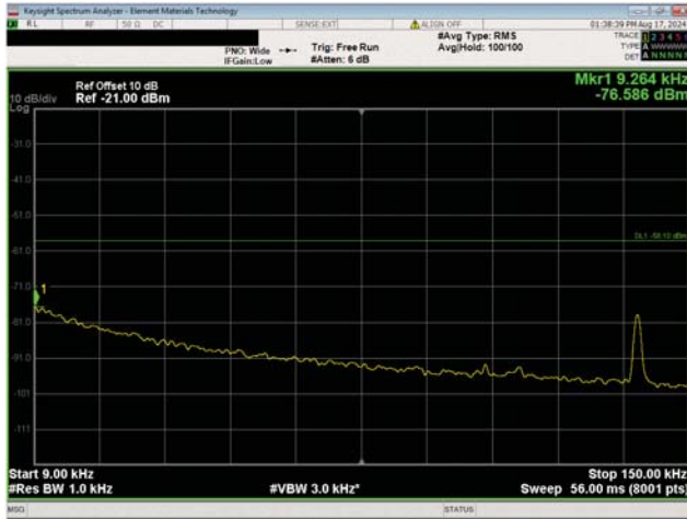
Port 1 10 MHz Channel Bandwidth QPSK Modulation Mid Channel, 3500.01 MHz
