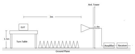
Radiated emission tests were performed in the 3 meters chamber test site, using the setup accordance with the ANSI C63.10-2013. The specification used was the FCC Part 15.209, FCC 15.247, RSS-Gen and RSS-247 Limits.
