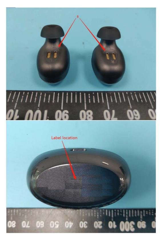
Conclusion: Based on the above description of area A to B, we conclude that the device is unquestionably too small for enabling the FCC certification No. to be printed onto any surface. We therefore request to move the FCC certification No. to the user's manual and charging case.
