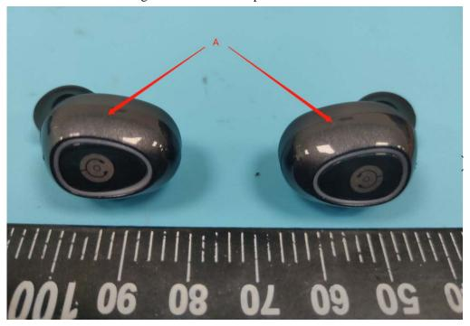
B. Top cover (B): The top cover does not provide enough physical space to fit the printing of the FCC certification No. according to below reference picture.
