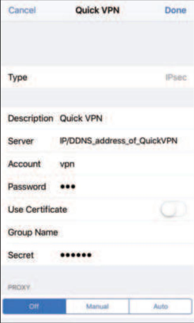
The screenshot shows the 'Quick VPN' configuration window on an iOS device. The window has a title bar with 'Cancel', 'Quick VPN', and 'Done' buttons. The configuration fields are as follows:
