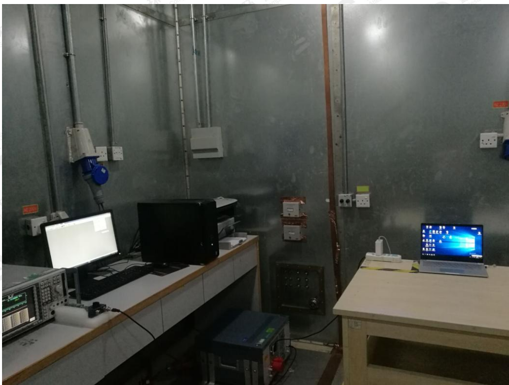
FCC RADIATED EMISSION TEST SETUP BELOW 1GHZ
