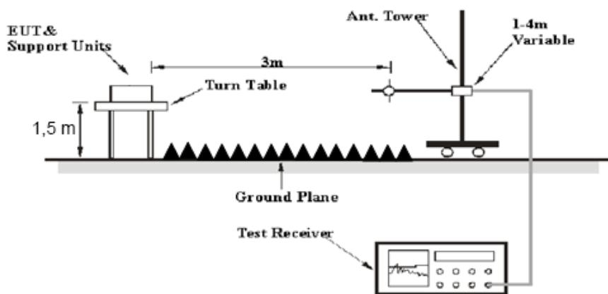
The radiated emission below 1GHz tests were performed in the 10 meters chamber test site, above 1GHz tests were performed in the 3 meters chamber test site A, using the setup accordance with the ANSI C63.10-2013. The specification used was the FCC 15.209, and FCC 15.247 limits and the RSS-247 Clause 5.5, RSS-GEN Clause 8.10 limits.
