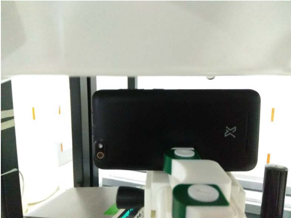
Body left side(separation distance is 10mm)
