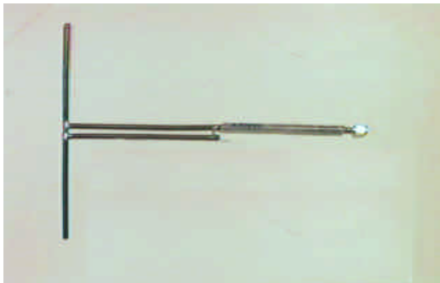
Reference Dipole Antenna Used for ERP Measurement
