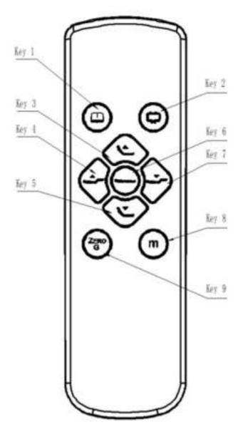
Key 1: Short press button 1, and the fader will run to a fixed position (Book mode) to stop; long press button 1, after 3 seconds, the current position will be memorized (overwrite the previous memory), the backlight will flash 3 times quickly, and the control box will beep
