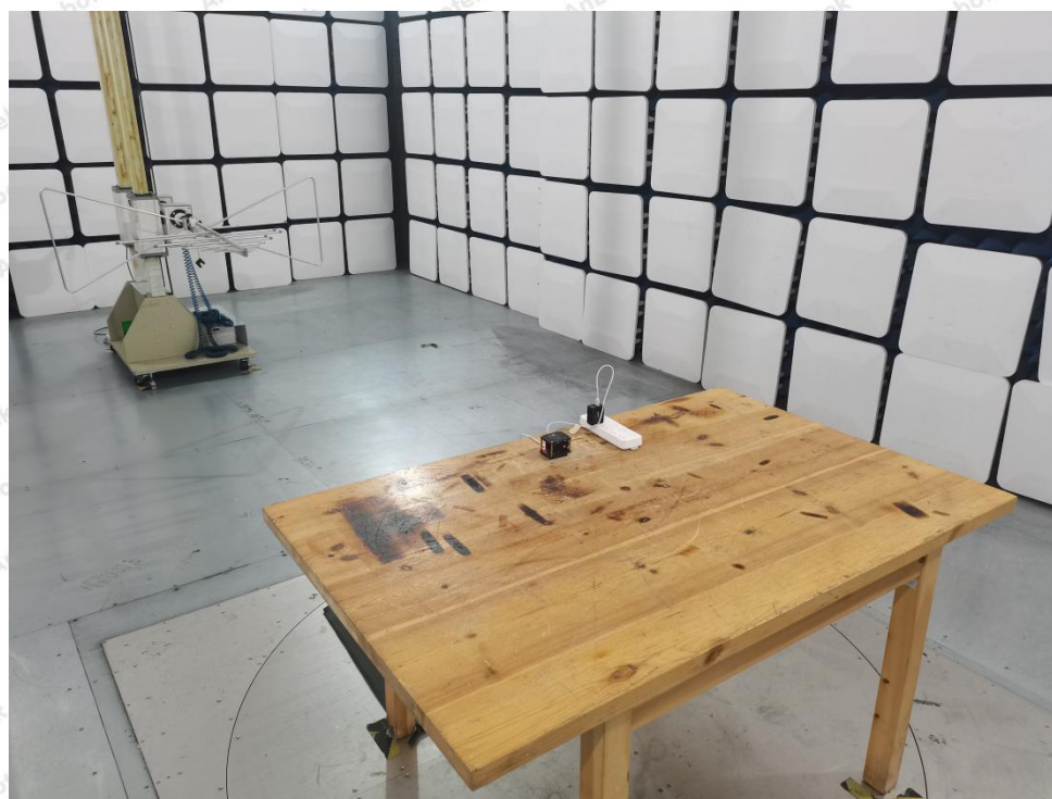
Photo of Radiation Emission Test
