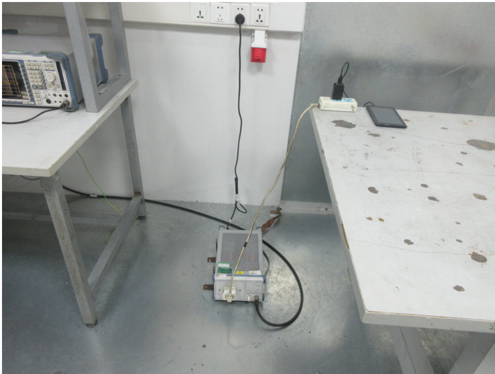
Photo of Conducted Emission Measurement
