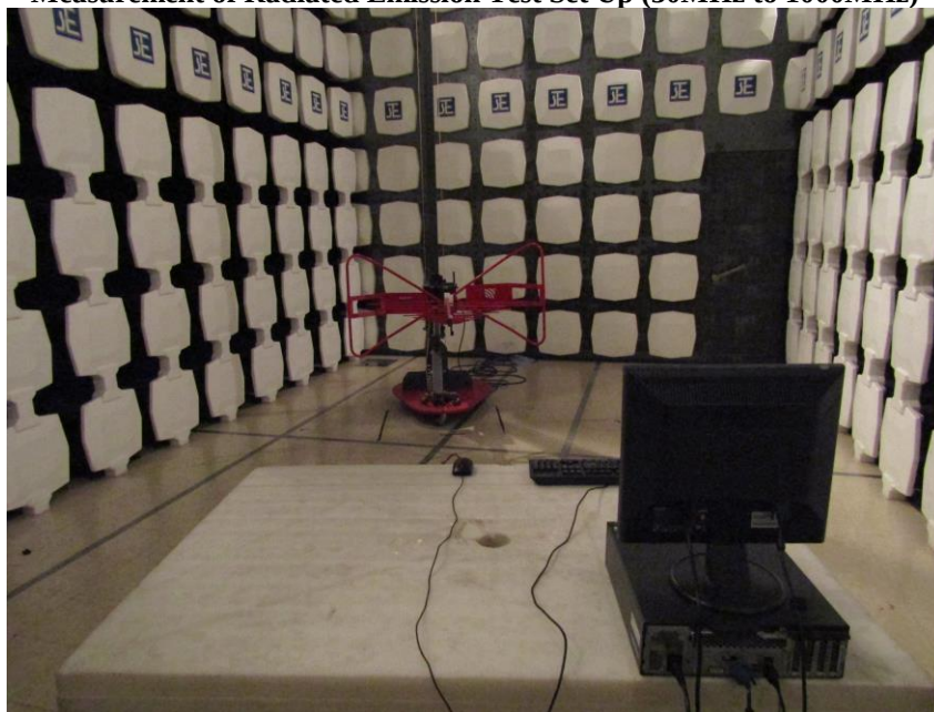
Measurement of Radiated Emission Test Set Up (30MHz to 1000MHz)
