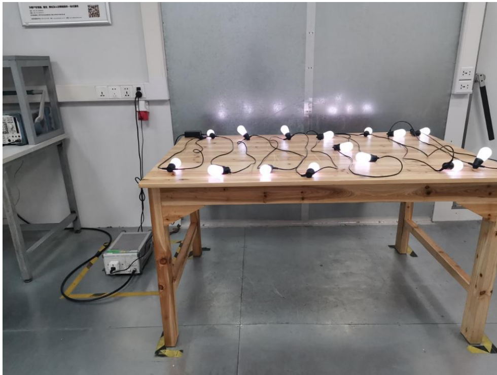
FCC ID: 2AQA6- H7002 Photo of Power Line Conducted Emission Test
