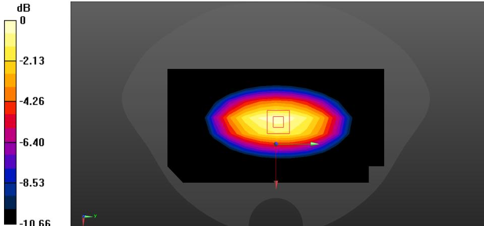
A 2D heatmap showing Specific Absorption Rate (SAR) distribution in a rectangular phantom section. The color scale on the left indicates SAR values in dB, ranging from -10.66 (dark blue) to 0 (yellow). The highest SAR values are concentrated in a central elliptical region, with a color gradient from red to yellow. A small square ROI is indicated in the center of the ellipse. A coordinate system (x, y) is shown at the bottom left.
