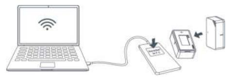
• Via TTL UART interface inside the device. Please select General type to log in ToolBox and configure the device. (Default password: **123456**)
