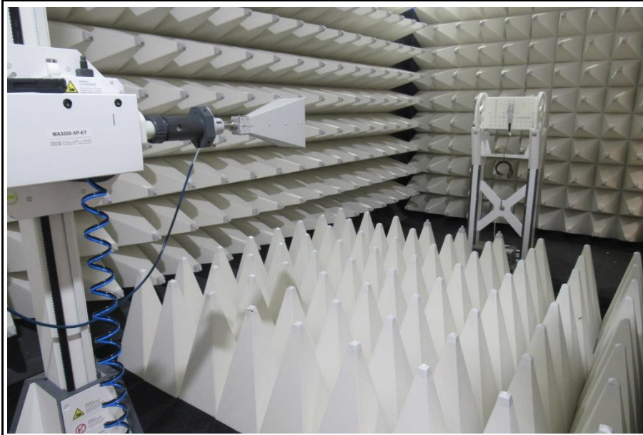
Setup for measurements above 1 GHz
