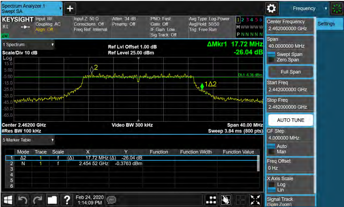
Figure 9: 6dB Bandwidth and 99% Bandwidth, 802.11n(HT20), 2462MHz
