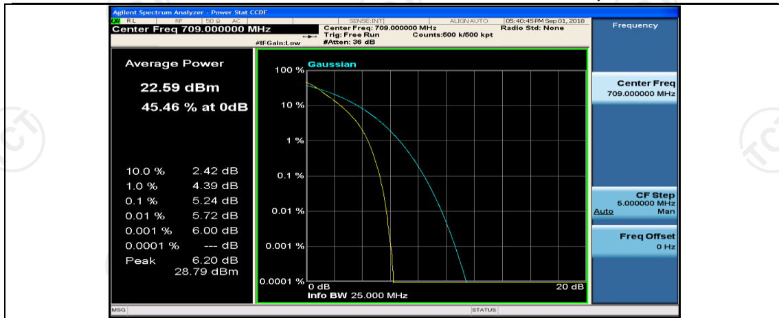
Channel Bandwidth: 10 MHz_MCH_QPSK_1RB#0
