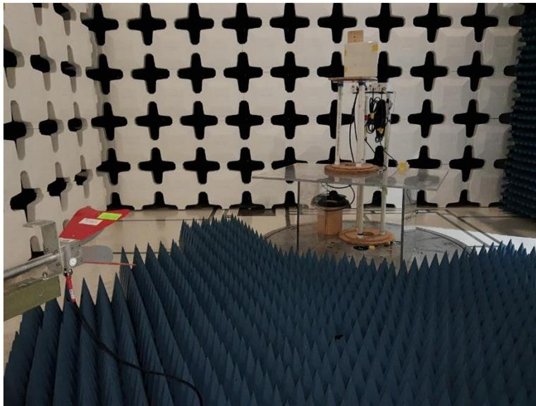
**Figure 4. Radiated Emissions Test Setup above 1GHz - 9.5dBi Antenna**
