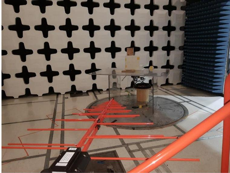
**Figure 7. Radiated Emissions Test Setup below 1GHz - 9.5dBi Antenna**
