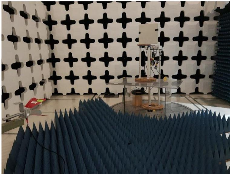
**Figure 2. Radiated Emissions Test Setup above 1GHz - 13dBi Antenna**
