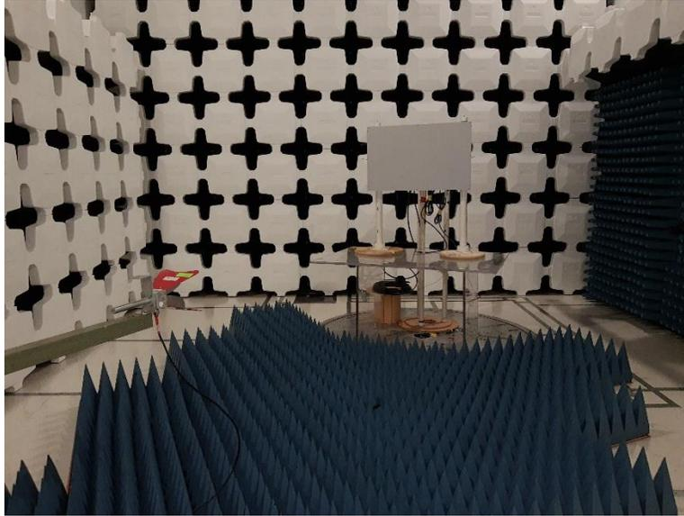
**Figure 3. Radiated Emissions Test Setup above 1GHz - 15dBi Antenna**
