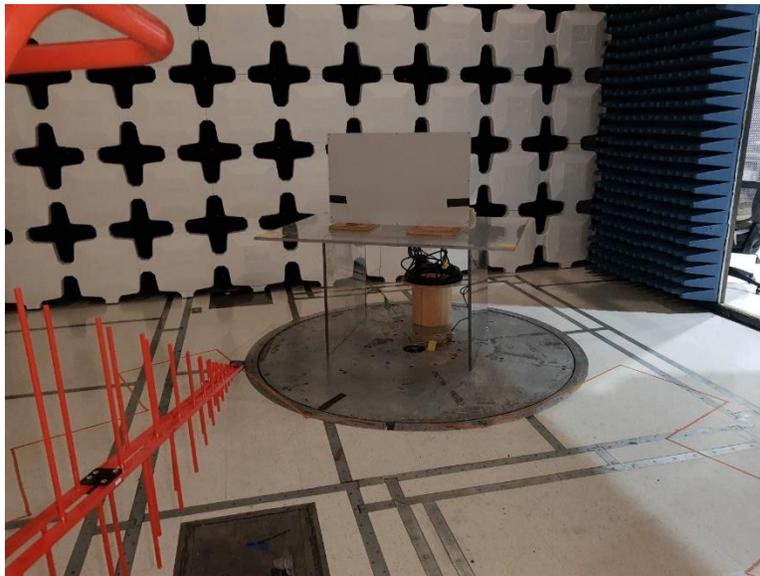
**Figure 6. Radiated Emissions Test Setup below 1GHz - 15dBi Antenna**
