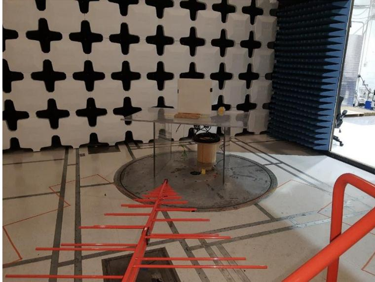
**Figure 5. Radiated Emissions Test Setup below 1GHz - 13dBi Antenna**
