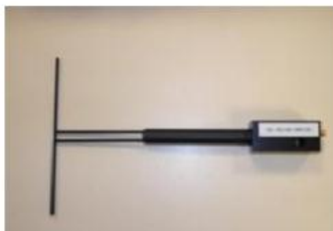
Figure 1 – Satimo COMOSAR Validation Dipole
