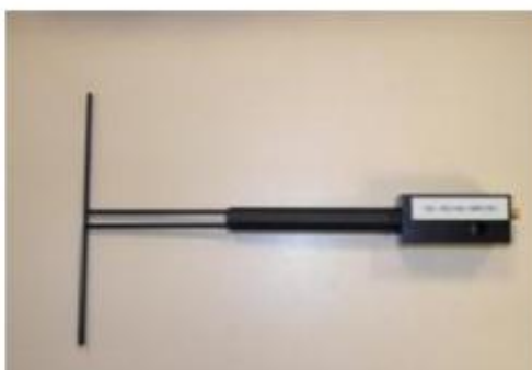
Figure 1 – Satimo COMOSAR Validation Dipole
