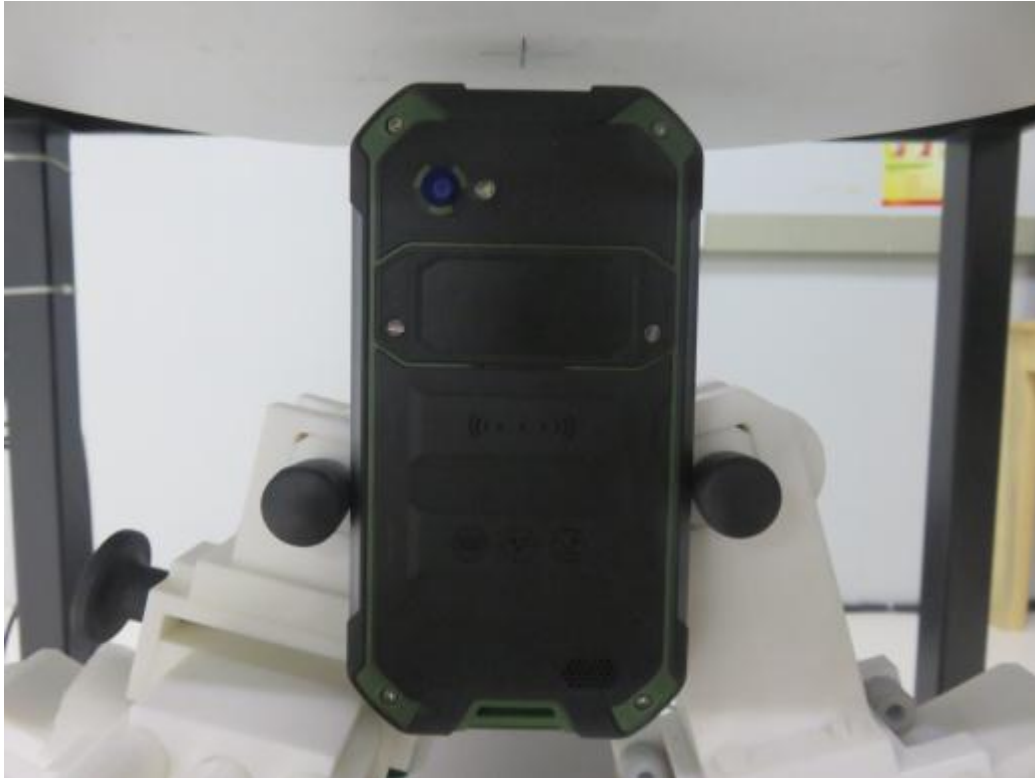
10mm body-worn Top Side Setup Photo(hotspot)
