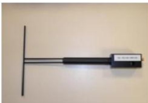
Figure 1 – Satimo COMOSAR Validation Dipole
