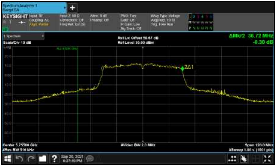
Figure 921 - Core 1 (B) 5755 MHz (CH151) 99% Bandwidth
