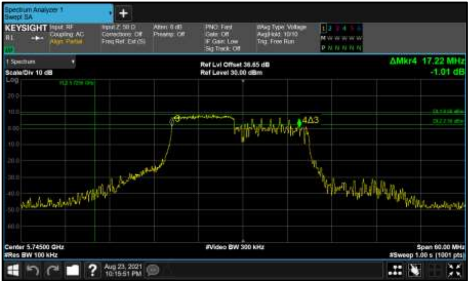
Figure 824 - Core 1 (B) 5745 MHz (CH149) 6 dB Bandwidth
