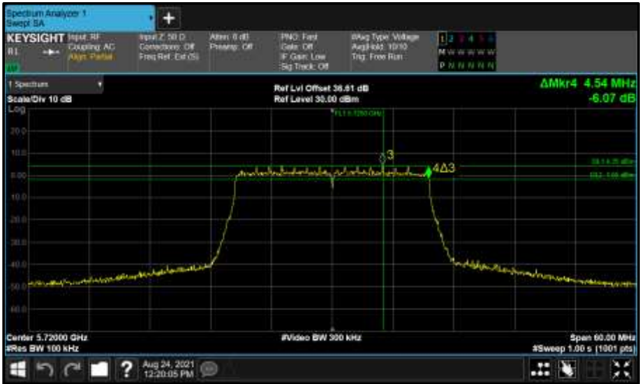
Figure 726 - Core 1 (B) 5720 MHz (CH144) 6 dB Bandwidth
