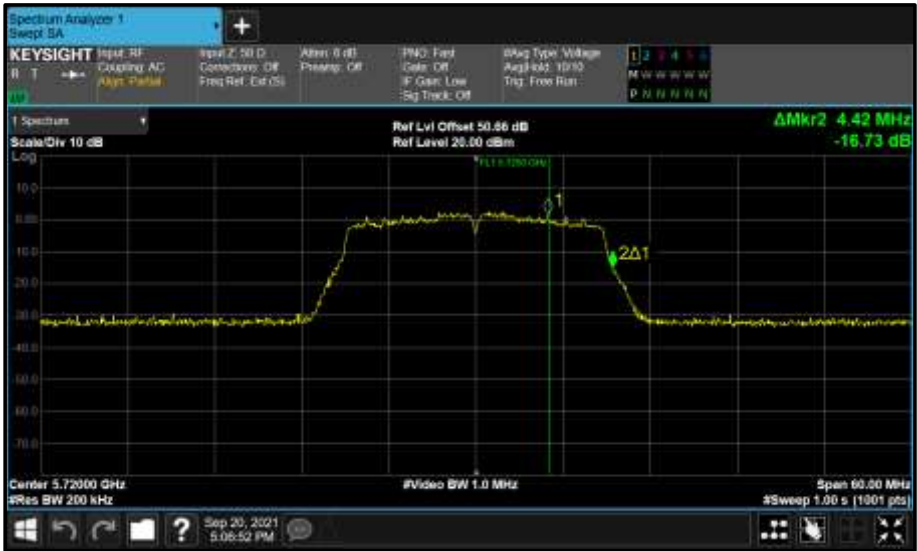
Figure 901 - Core 1 (B) 5720 MHz (CH144) 99% Bandwidth
