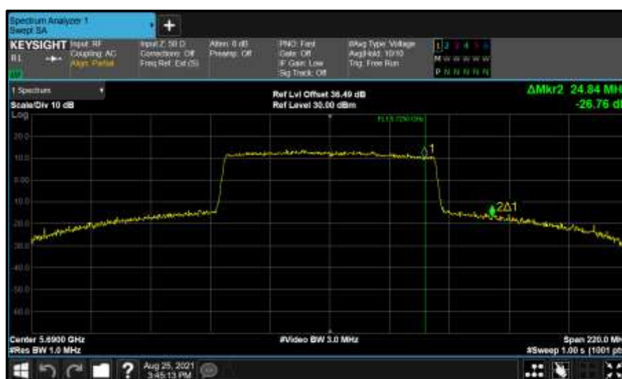
Figure 879 - Core 1 (B) 5690 MHz (CH138) 99% Bandwidth
