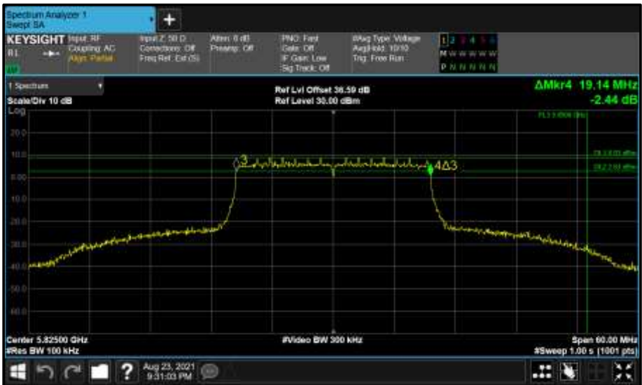
Figure 706 - Core 1 (B) 5825 MHz (CH165) 6 dB Bandwidth
