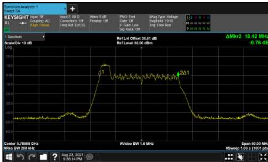
Figure 741 - Core 1 (B) 5785 MHz (CH157) 99% Bandwidth
