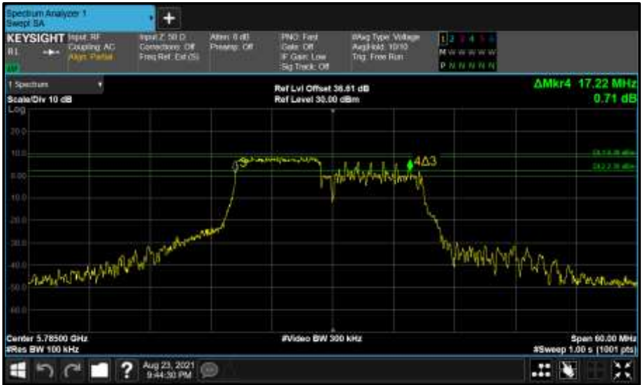
Figure 814 - Core 1 (B) 5785 MHz (CH157) 6 dB Bandwidth
