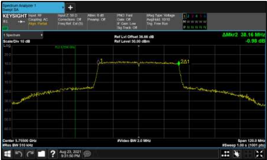
Figure 851 - Core 1 (B) 5755 MHz (CH151) 99% Bandwidth
