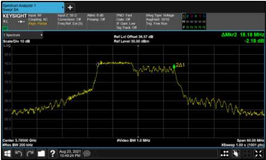
Figure 841 - Core 0 (A) 5785 MHz (CH157) 99% Bandwidth
