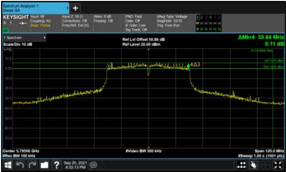
Figure 926 - Core 1 (B) 5795 MHz (CH159) 6 dB Bandwidth
