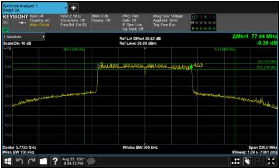
Figure 882 - Core 1 (B) 5775 MHz (CH155) 6 dB Bandwidth
