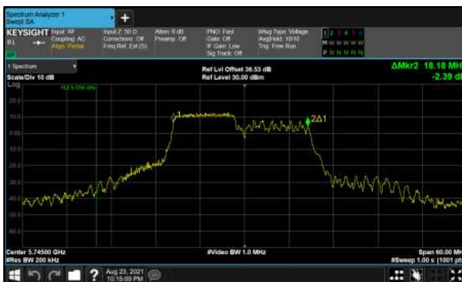
Figure 821 - Core 0 (A) 5745 MHz (CH149) 99% Bandwidth
