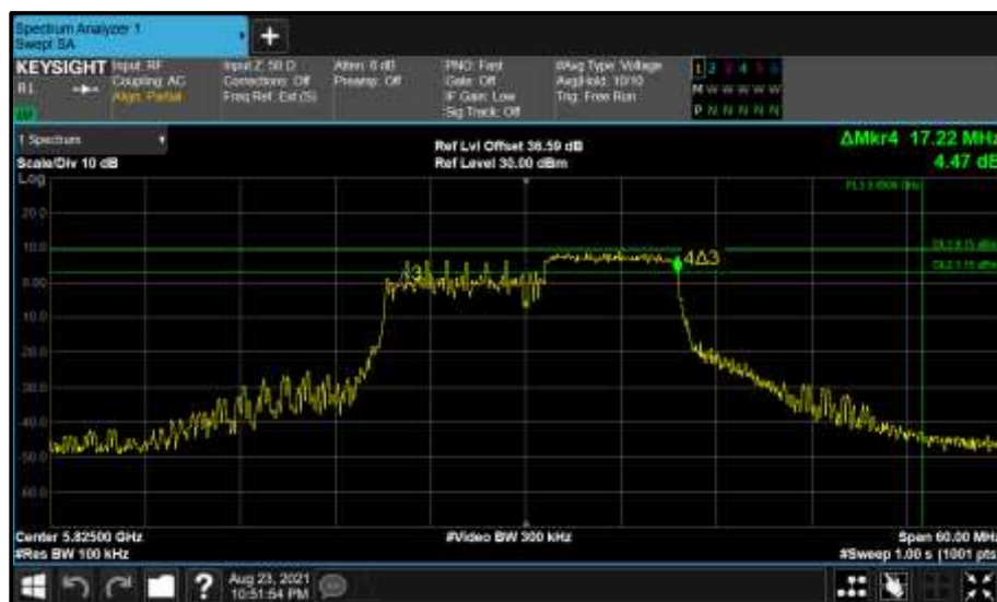
Figure 848 - Core 1 (B) 5825 MHz (CH165) 6 dB Bandwidth
