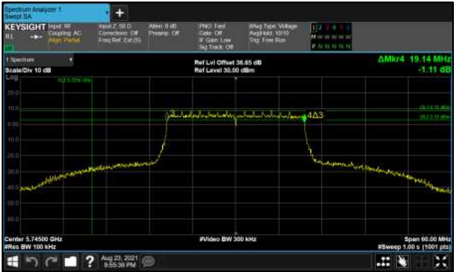
Figure 714 - Core 1 (B) 5745 MHz (CH149) 6 dB Bandwidth
