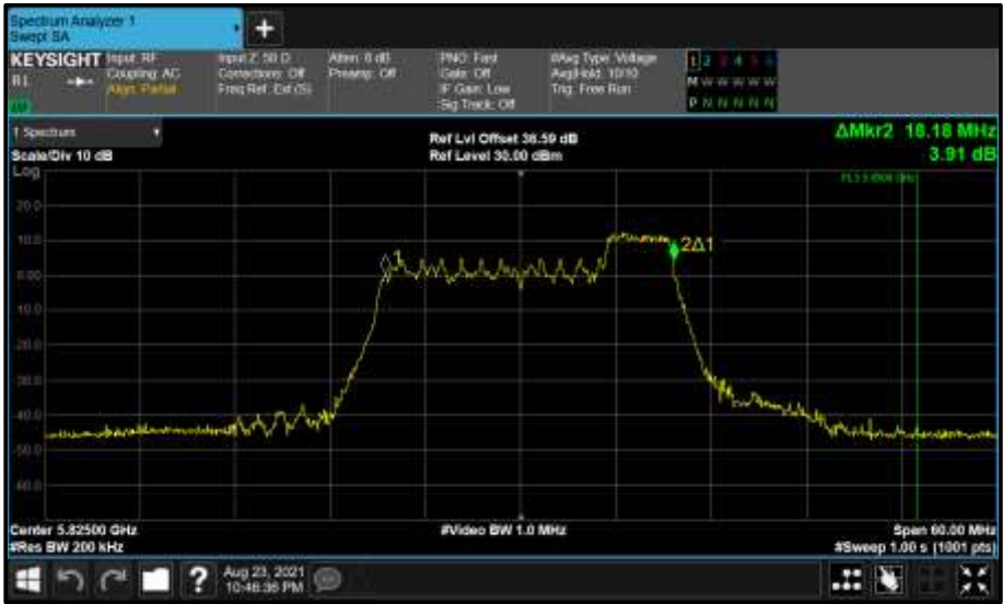
Figure 807 - Core 1 (B) 5825 MHz (CH165) 99% Bandwidth
