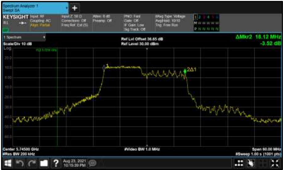
Figure 823 - Core 1 (B) 5745 MHz (CH149) 99% Bandwidth
