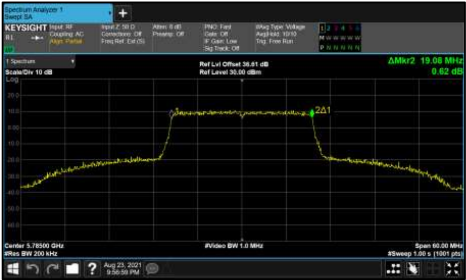
Figure 717 - Core 1 (B) 5785 MHz (CH157) 99% Bandwidth
