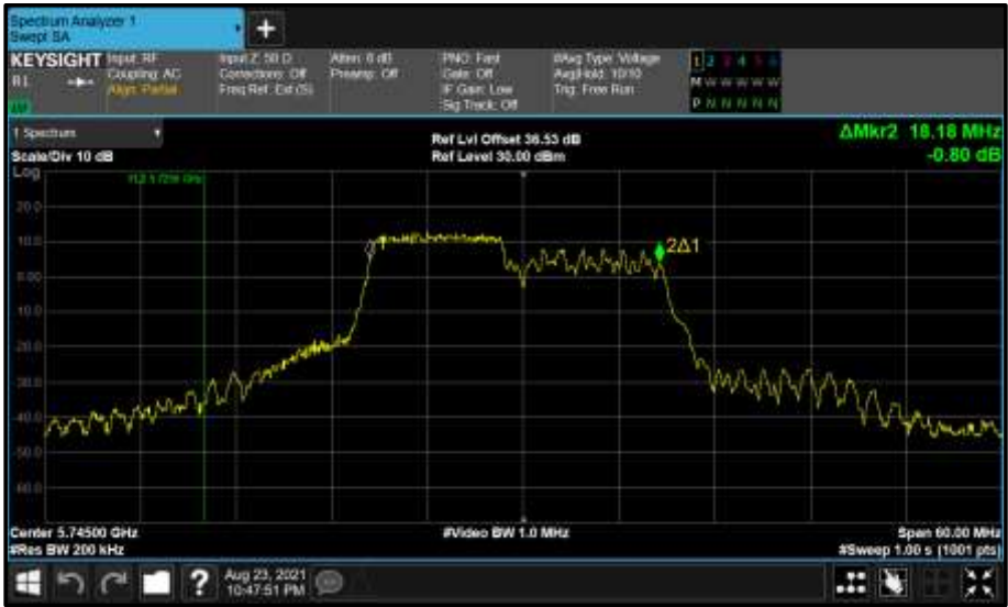
Figure 837 - Core 0 (A) 5745 MHz (CH149) 99% Bandwidth
