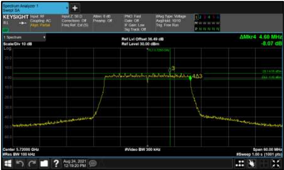
Figure 724 - Core 0 (A) 5720 MHz (CH144) 6 dB Bandwidth
