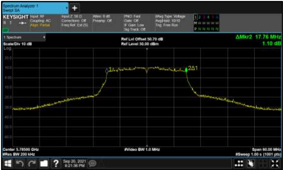
Figure 907 - Core 0 (A) 5785 MHz (CH157) 99% Bandwidth
