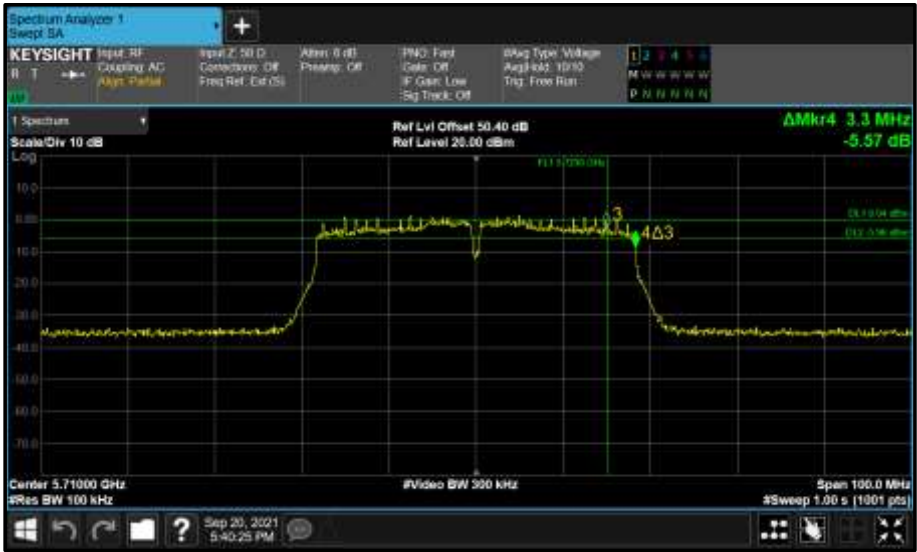
Figure 916 - Core 0 (A) 5710 MHz (CH142) 6 dB Bandwidth
