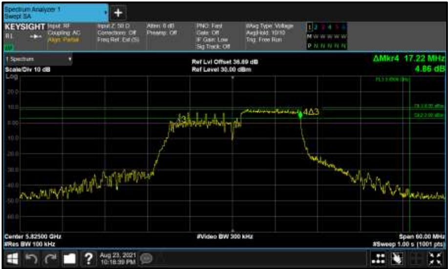
Figure 830 - Core 0 (A) 5825 MHz (CH165) 6 dB Bandwidth
