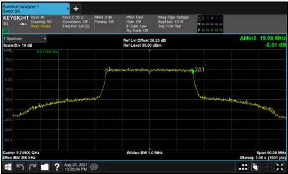
Figure 727 - Core 0 (A) 5745 MHz (CH149) 99% Bandwidth
