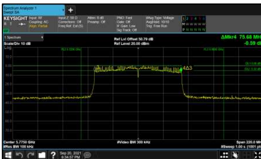
Figure 934 - Core 1 (B) 5775 MHz (CH155) 6 dB Bandwidth
