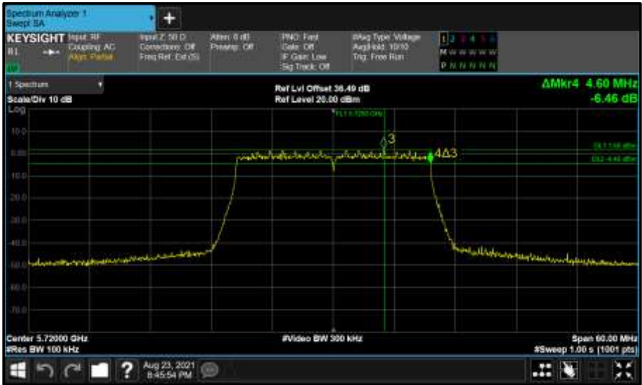
Figure 708 - Core 0 (A) 5720 MHz (CH144) 6 dB Bandwidth
