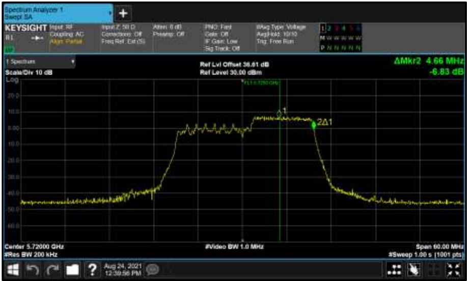
Figure 835 - Core 1 (B) 5720 MHz (CH144) 99% Bandwidth
