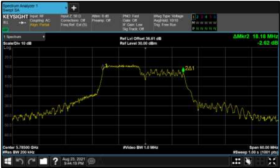
Figure 813 - Core 1 (B) 5785 MHz (CH157) 99% Bandwidth
