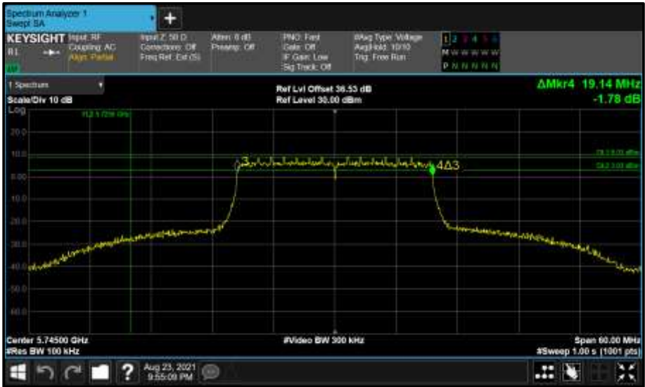
Figure 712 - Core 0 (A) 5745 MHz (CH149) 6 dB Bandwidth
