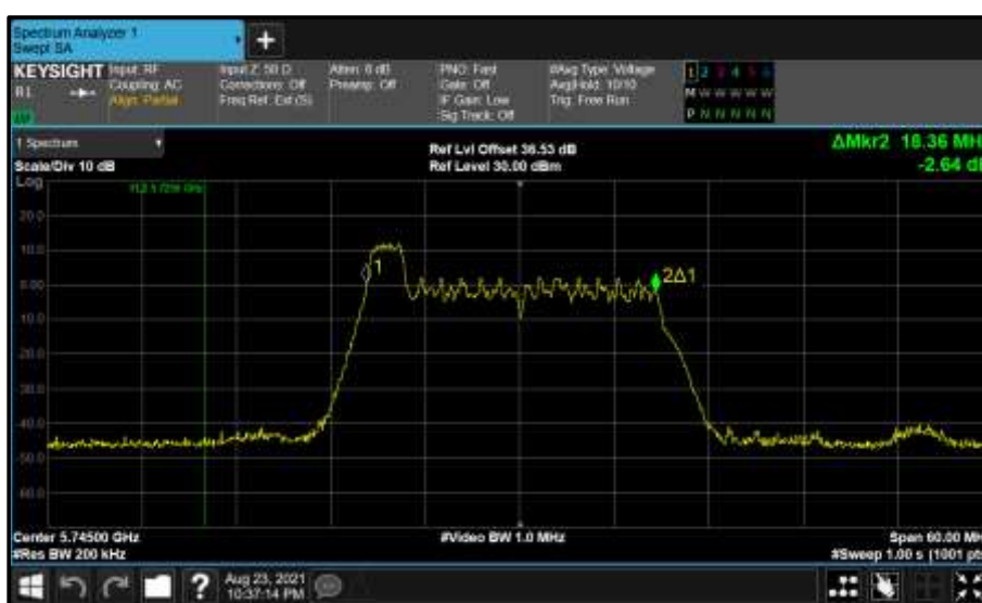
Figure 757 - Core 0 (A) 5745 MHz (CH149) 99% Bandwidth
