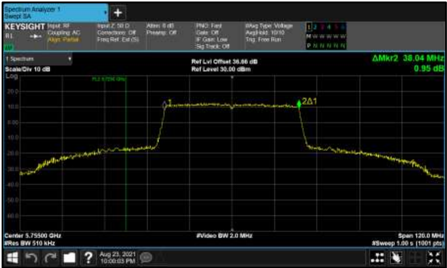
Figure 861 - Core 1 (B) 5755 MHz (CH151) 99% Bandwidth
