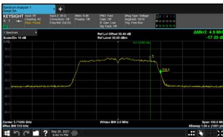
Figure 915 - Core 0 (A) 5710 MHz (CH142) 99% Bandwidth
