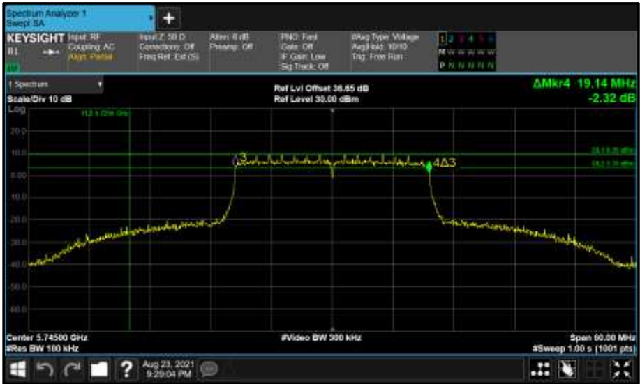
Figure 702 - Core 1 (B) 5745 MHz (CH149) 6 dB Bandwidth
