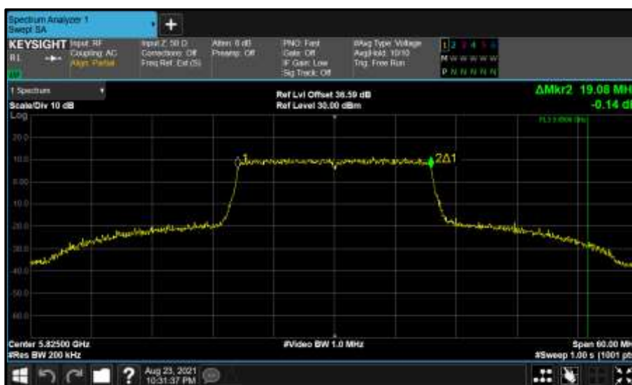
Figure 737 - Core 1 (B) 5825 MHz (CH165) 99% Bandwidth
