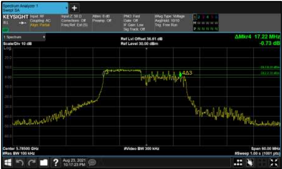
Figure 828 - Core 1 (B) 5785 MHz (CH157) 6 dB Bandwidth
