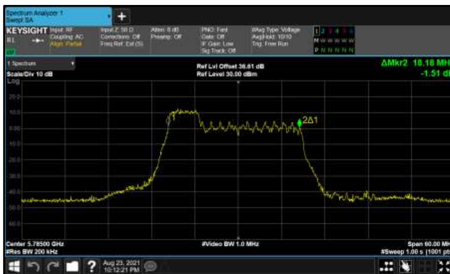
Figure 787 - Core 1 (B) 5785 MHz (CH157) 99% Bandwidth
