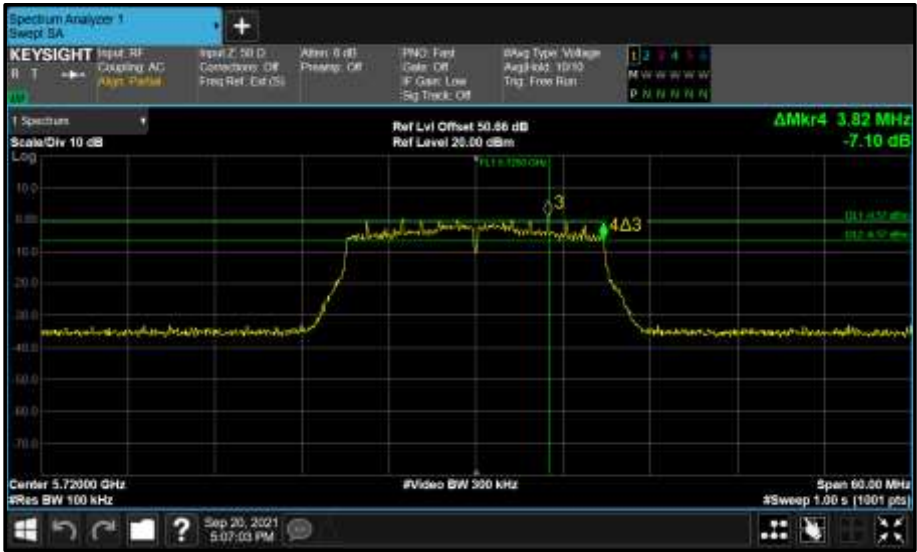
Figure 902 - Core 1 (B) 5720 MHz (CH144) 6 dB Bandwidth
