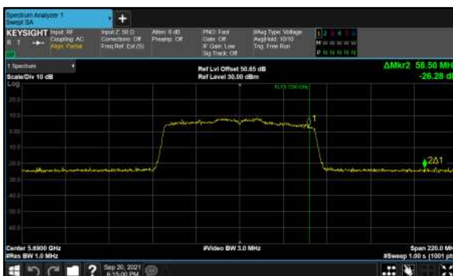
Figure 929 - Core 1 (B) 5690 MHz (CH138) 99% Bandwidth
