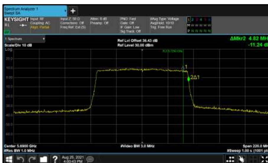
Figure 883 - Core 0 (A) 5690 MHz (CH138) 99% Bandwidth
