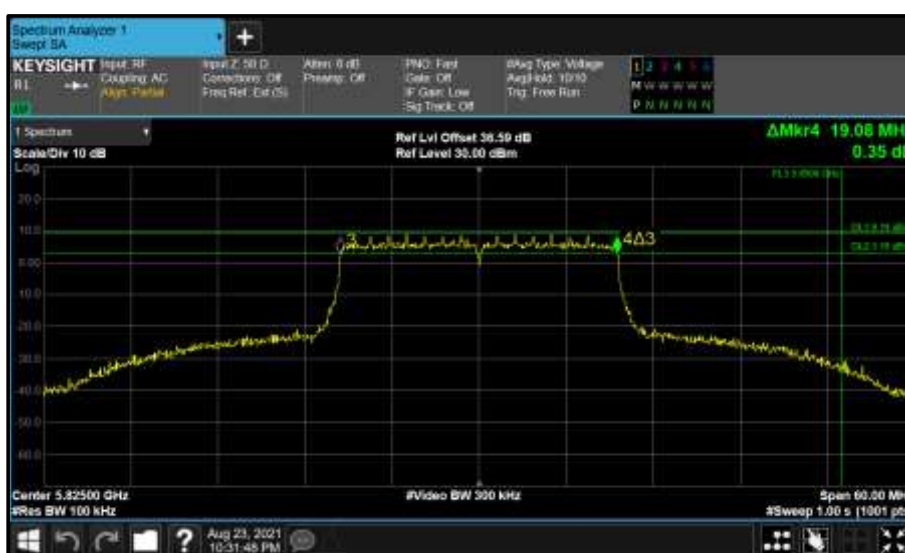
Figure 738 - Core 1 (B) 5825 MHz (CH165) 6 dB Bandwidth
