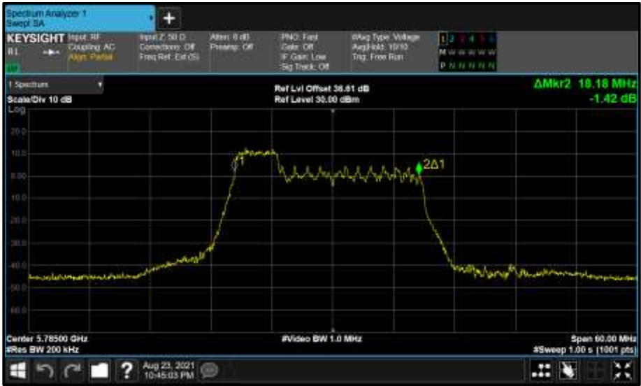
Figure 803 - Core 1 (B) 5785 MHz (CH157) 99% Bandwidth
