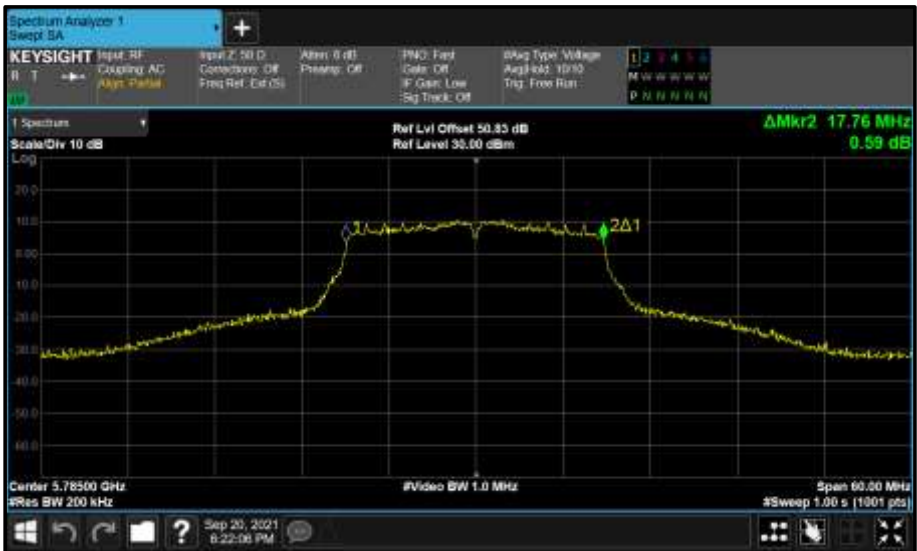
Figure 909 - Core 1 (B) 5785 MHz (CH157) 99% Bandwidth
