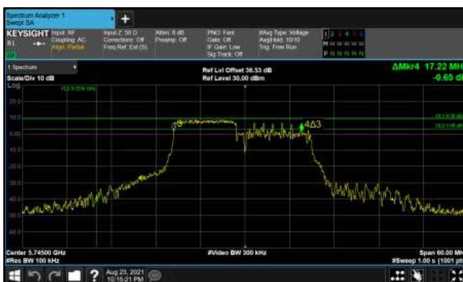
Figure 822 - Core 0 (A) 5745 MHz (CH149) 6 dB Bandwidth
