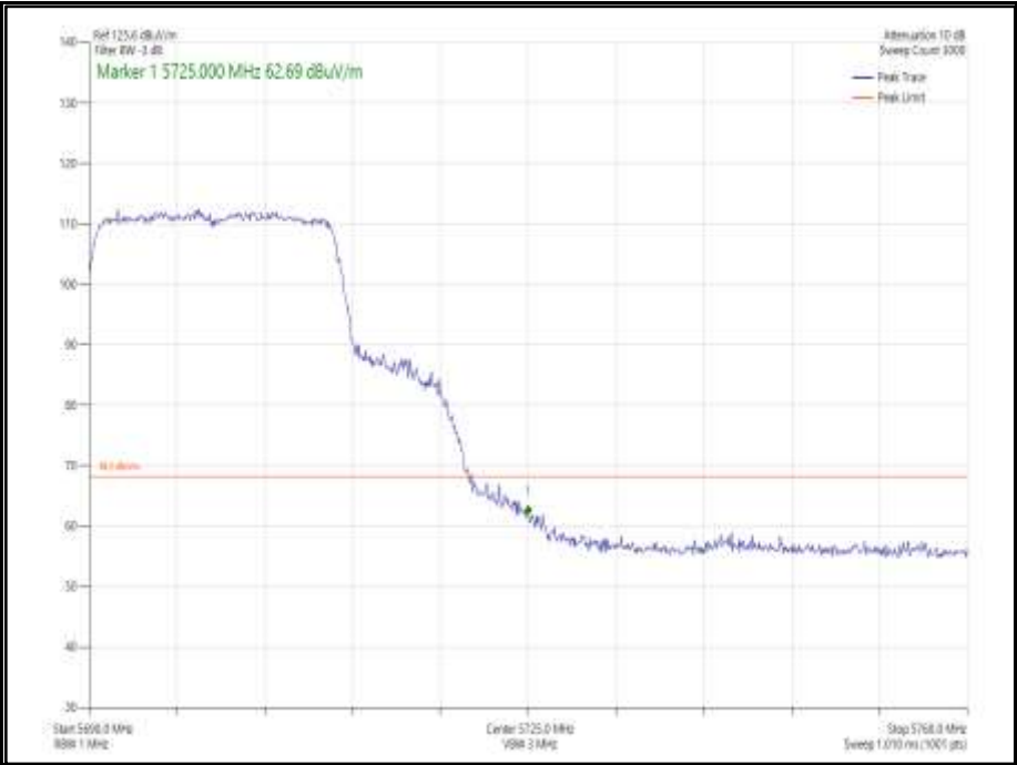
Figure 941- 802.11ax HE20, Core 1, SU - 5700 MHz Band Edge Frequency 5725 MHz
