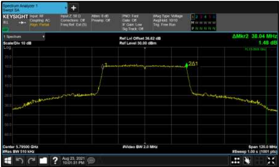
Figure 865 - Core 1 (B) 5795 MHz (CH159) 99% Bandwidth
