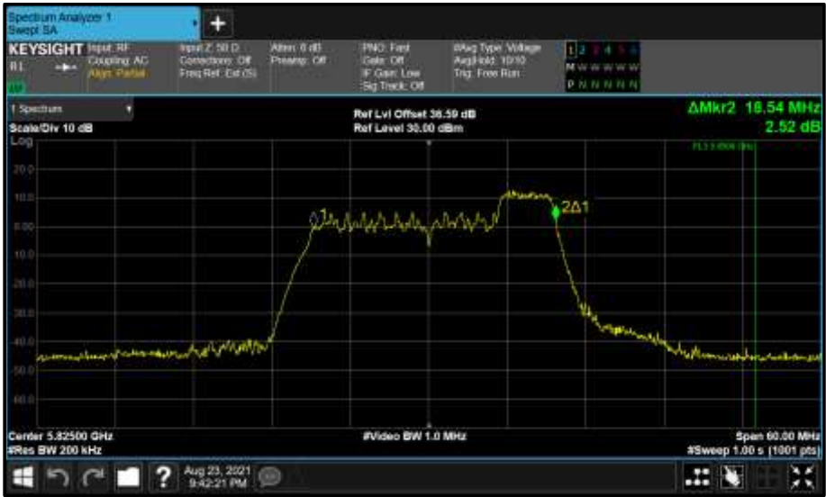
Figure 775 - Core 1 (B) 5825 MHz (CH165) 99% Bandwidth
