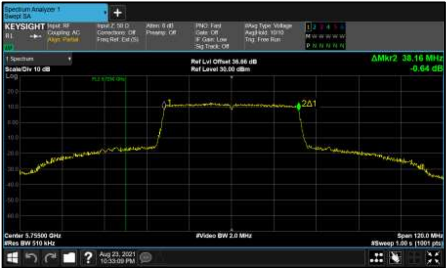
Figure 873 - Core 1 (B) 5755 MHz (CH151) 99% Bandwidth
