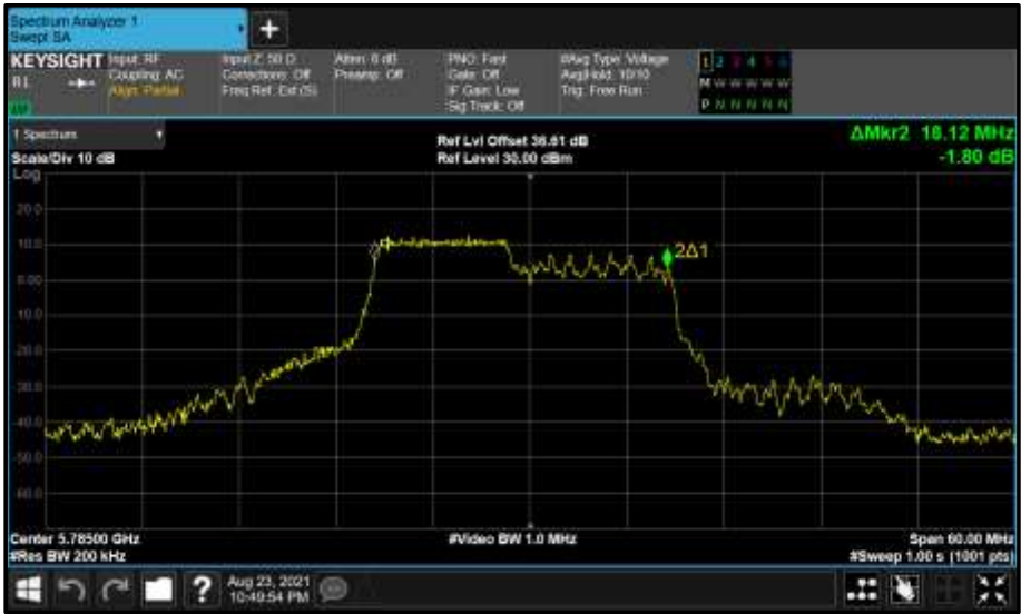
Figure 843 - Core 1 (B) 5785 MHz (CH157) 99% Bandwidth
