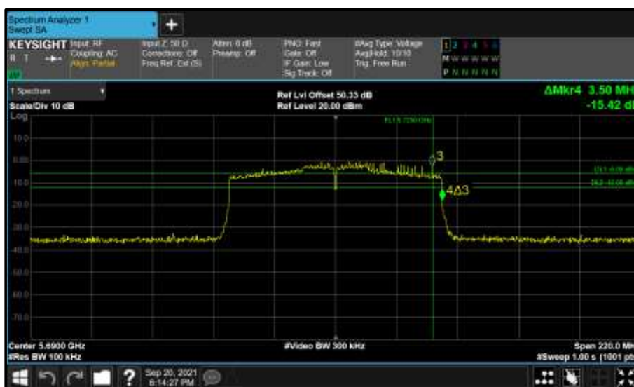
Figure 928 - Core 0 (A) 5690 MHz (CH138) 6 dB Bandwidth
