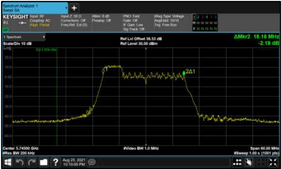
Figure 781 - Core 0 (A) 5745 MHz (CH149) 99% Bandwidth
