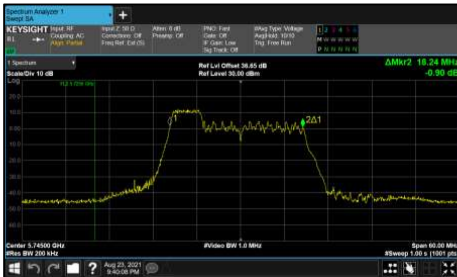
Figure 771 - Core 1 (B) 5745 MHz (CH149) 99% Bandwidth
