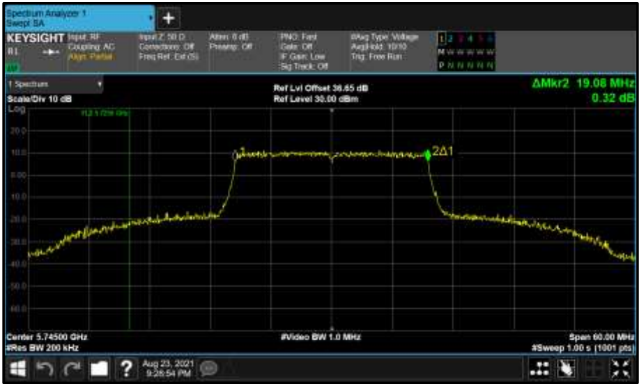
Figure 701 - Core 1 (B) 5745 MHz (CH149) 99% Bandwidth
