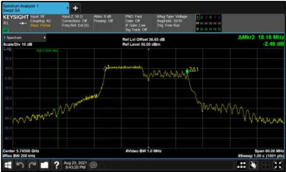
Figure 811 - Core 1 (B) 5745 MHz (CH149) 99% Bandwidth
