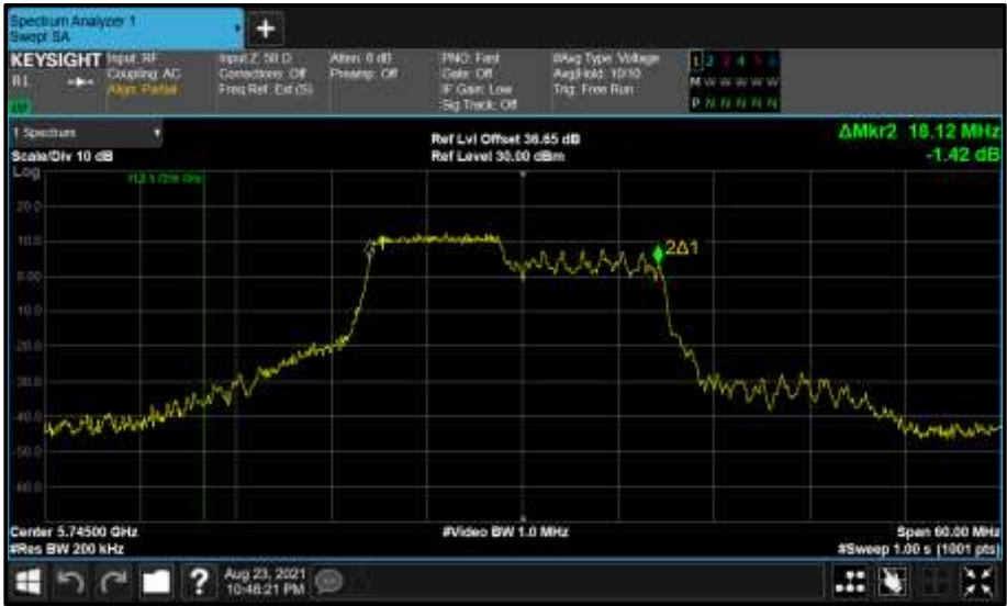
Figure 839 - Core 1 (B) 5745 MHz (CH149) 99% Bandwidth
