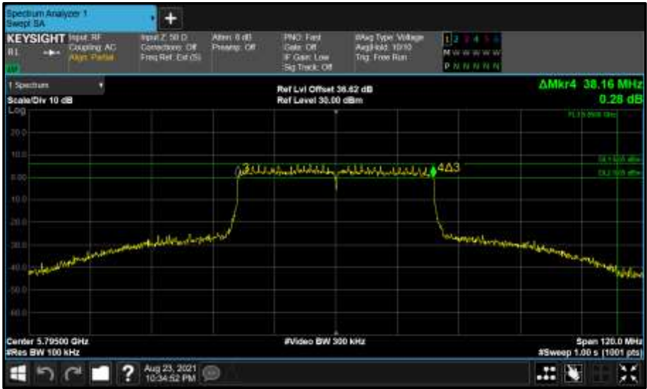
Figure 878 - Core 1 (B) 5795 MHz (CH159) 6 dB Bandwidth
