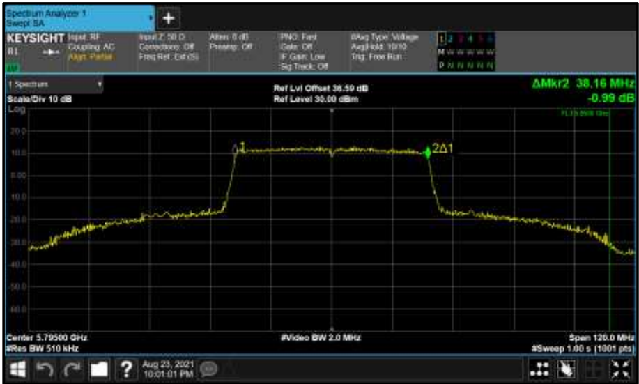
Figure 863 - Core 0 (A) 5795 MHz (CH159) 99% Bandwidth
