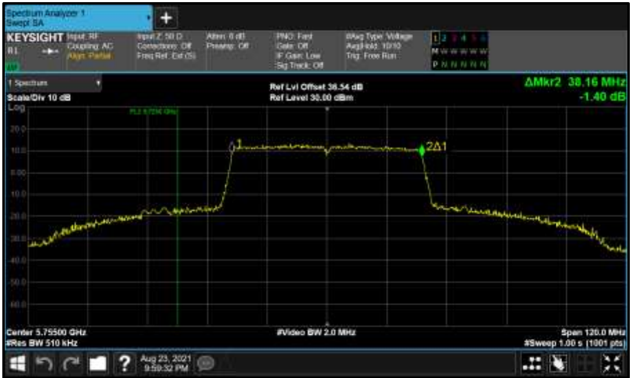
Figure 859 - Core 0 (A) 5755 MHz (CH151) 99% Bandwidth
