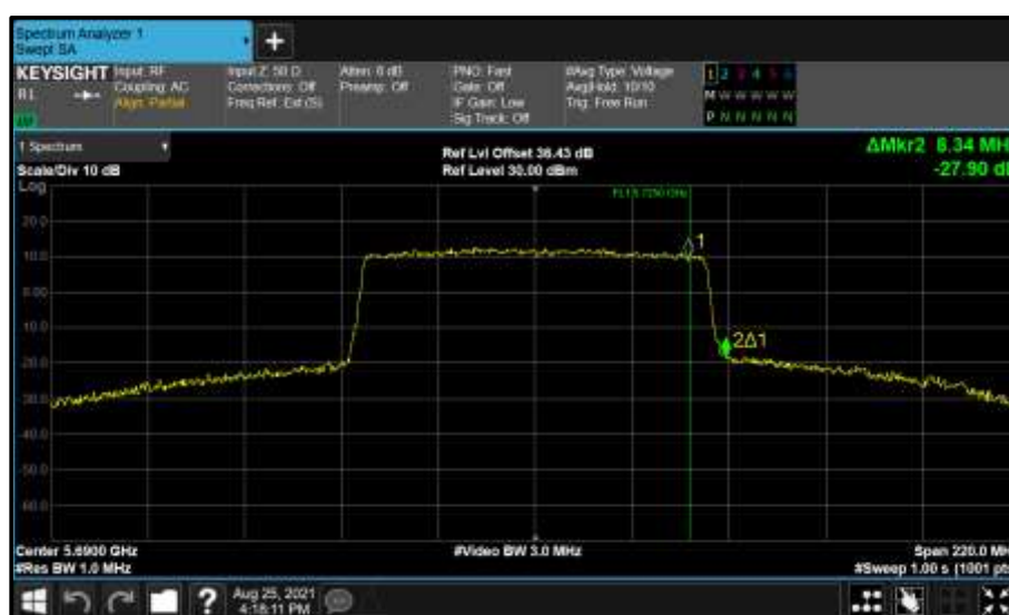
Figure 891 - Core 0 (A) 5690 MHz (CH138) 99% Bandwidth
