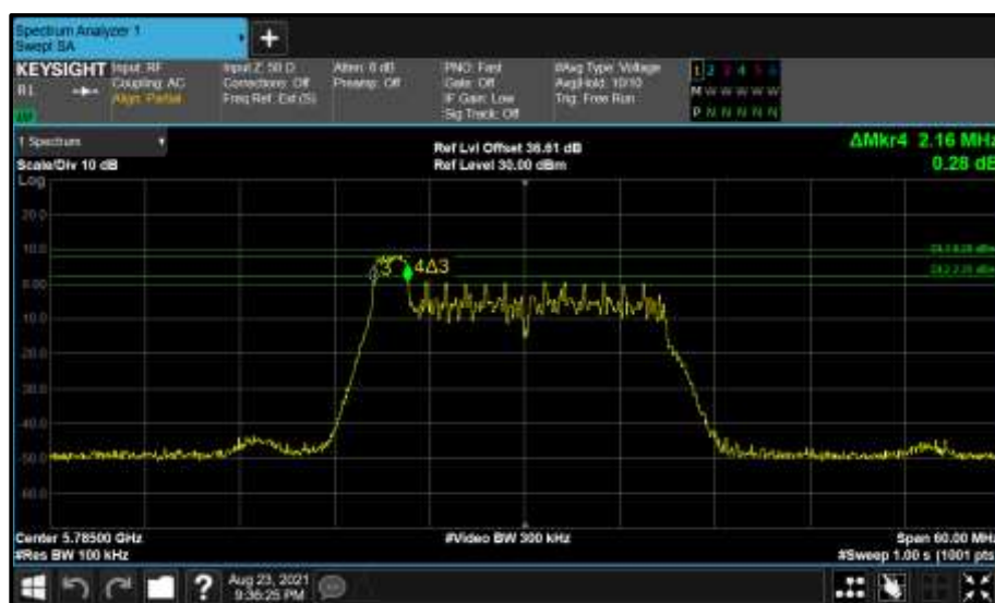
Figure 742 - Core 1 (B) 5785 MHz (CH157) 6 dB Bandwidth
