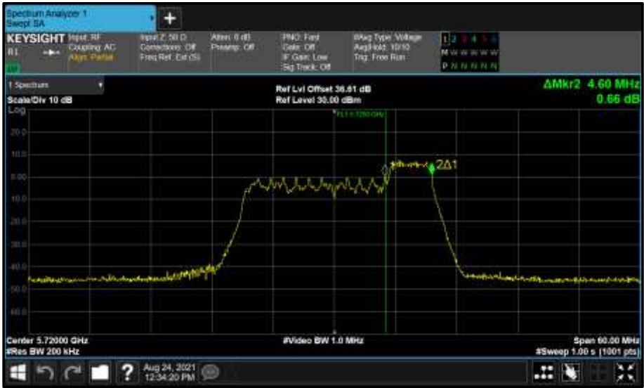
Figure 795 - Core 1 (B) 5720 MHz (CH144) 99% Bandwidth
