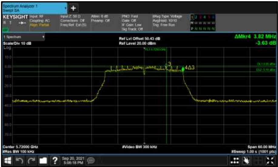
Figure 900 - Core 0 (A) 5720 MHz (CH144) 6 dB Bandwidth
