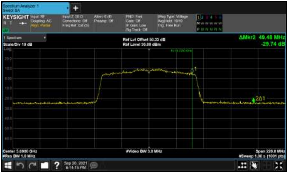
Figure 927 - Core 0 (A) 5690 MHz (CH138) 99% Bandwidth
