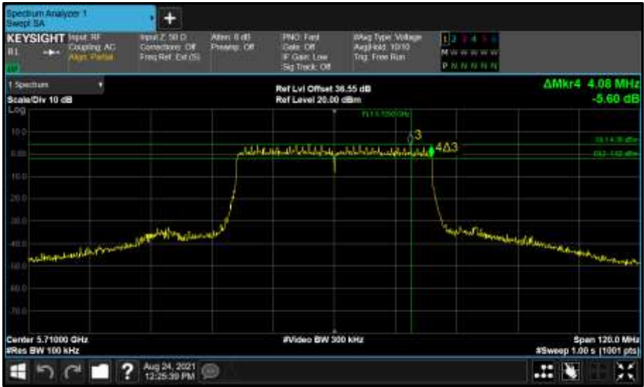
Figure 870 - Core 1 (B) 5710 MHz (CH142) 6 dB Bandwidth
