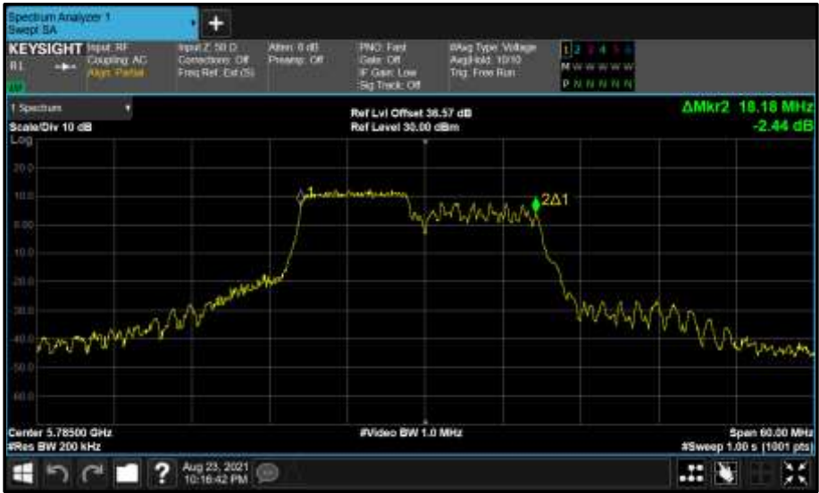
Figure 825 - Core 0 (A) 5785 MHz (CH157) 99% Bandwidth
