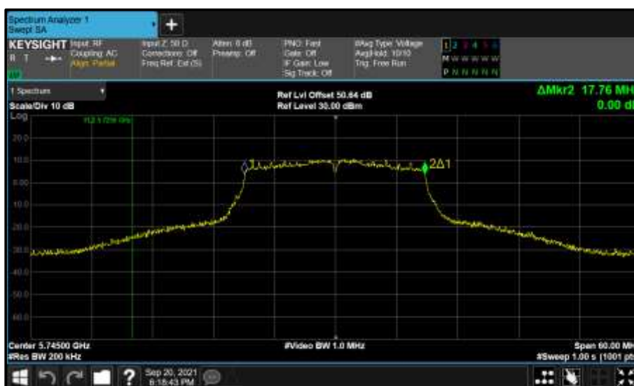
Figure 905 - Core 1 (B) 5745 MHz (CH149) 99% Bandwidth
