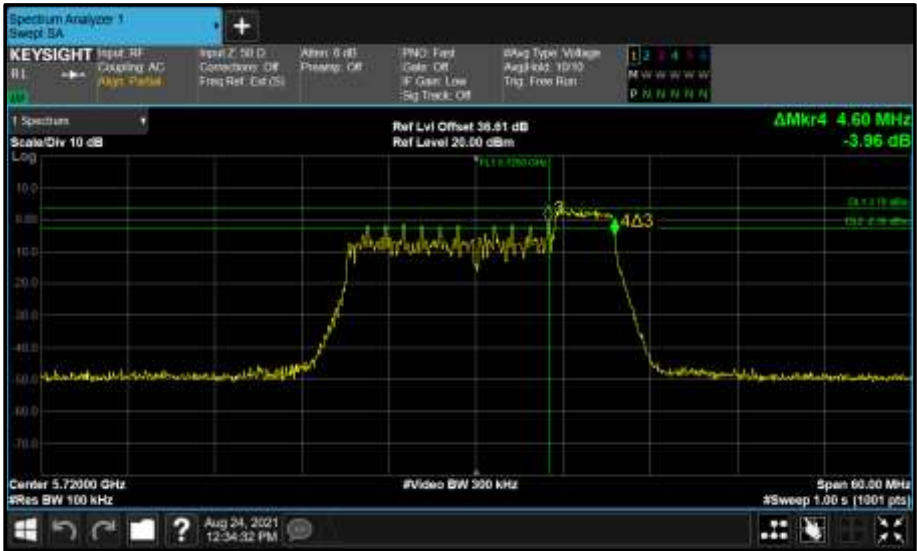
Figure 796 - Core 1 (B) 5720 MHz (CH144) 6 dB Bandwidth
