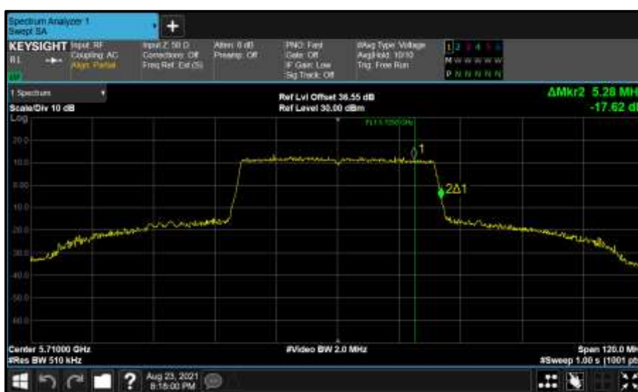
Figure 849 - Core 1 (B) 5710 MHz (CH142) 99% Bandwidth
