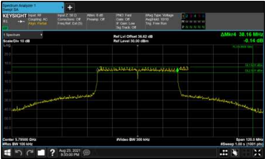
Figure 854 - Core 1 (B) 5795 MHz (CH159) 6 dB Bandwidth
