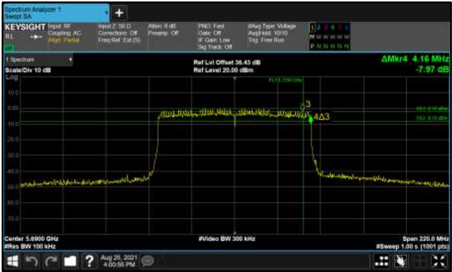
Figure 884 - Core 0 (A) 5690 MHz (CH138) 6 dB Bandwidth
