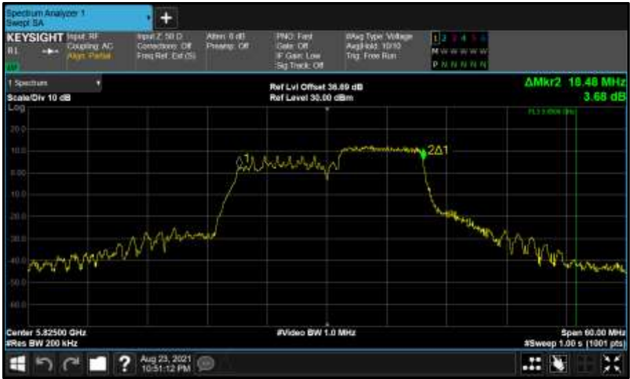
Figure 845 - Core 0 (A) 5825 MHz (CH165) 99% Bandwidth
