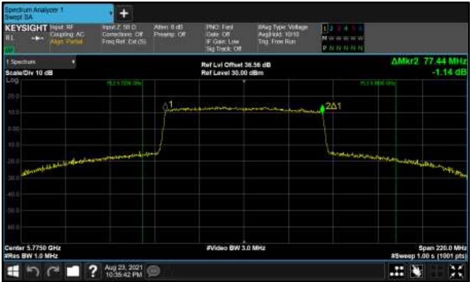
Figure 895 - Core 0 (A) 5775 MHz (CH155) 99% Bandwidth
