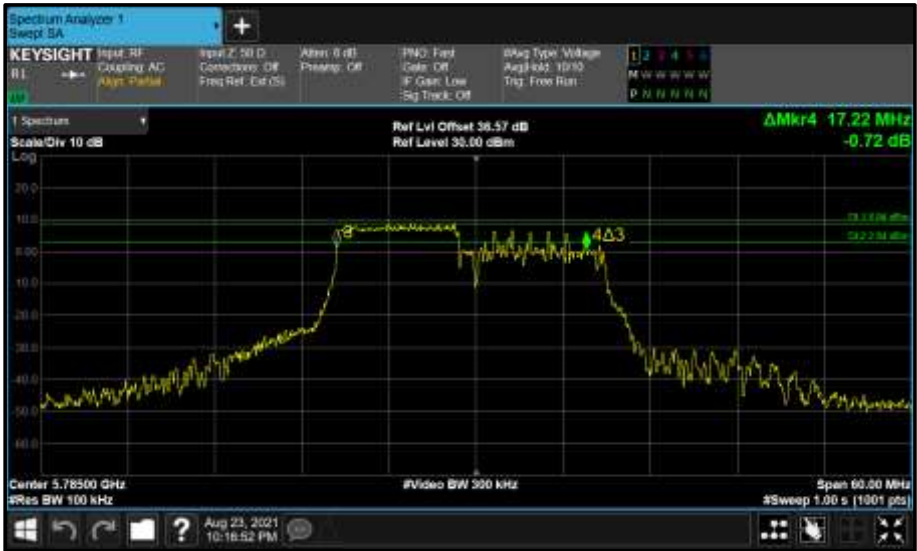
Figure 826 - Core 0 (A) 5785 MHz (CH157) 6 dB Bandwidth
