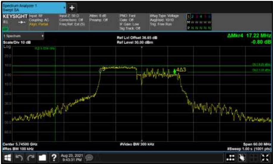
Figure 812 - Core 1 (B) 5745 MHz (CH149) 6 dB Bandwidth
