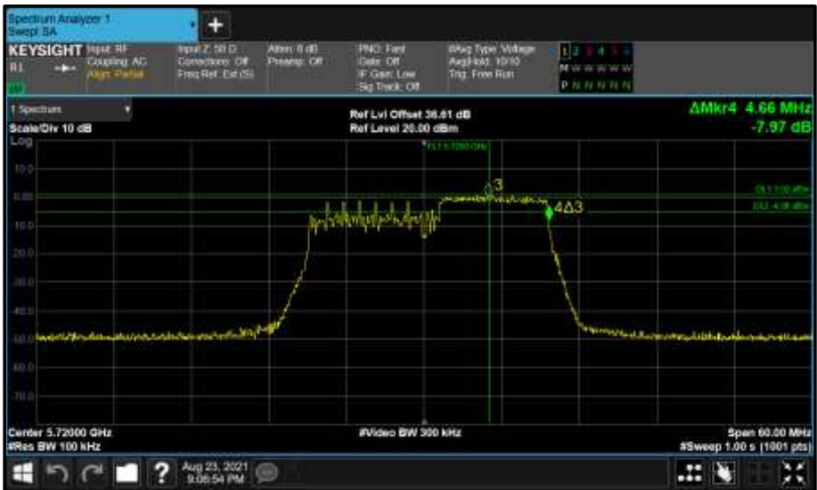
Figure 820 - Core 1 (B) 5720 MHz (CH144) 6 dB Bandwidth
