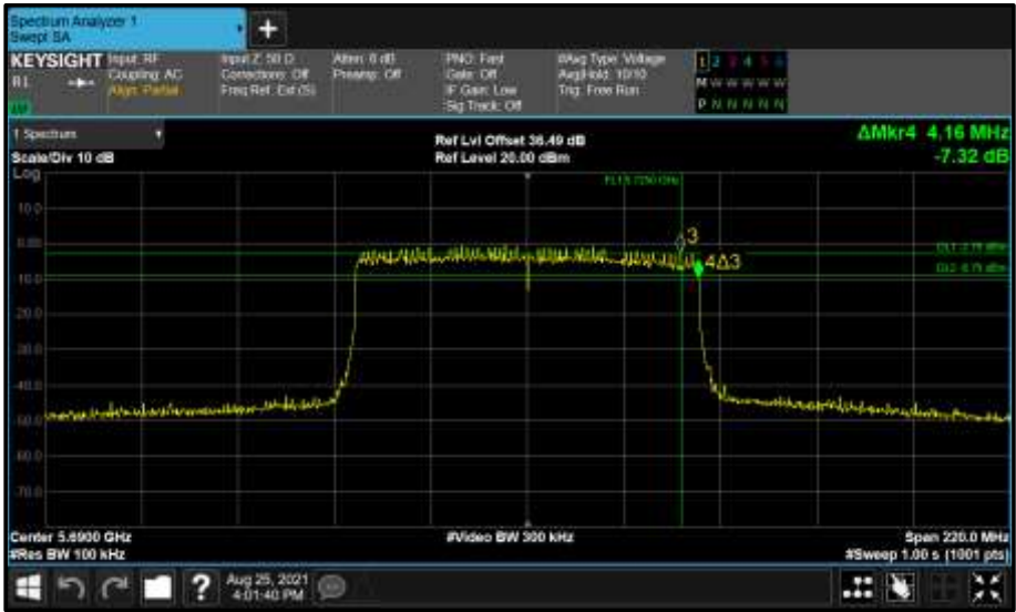
Figure 886 - Core 1 (B) 5690 MHz (CH138) 6 dB Bandwidth
