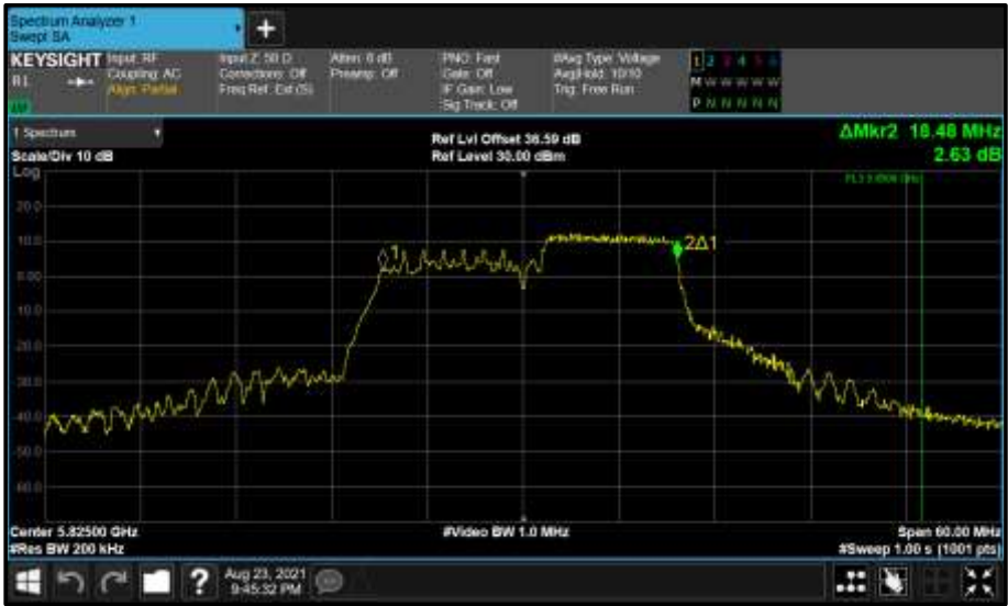
Figure 815 - Core 1 (B) 5825 MHz (CH165) 99% Bandwidth
