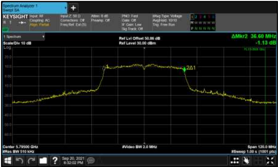
Figure 925 - Core 1 (B) 5795 MHz (CH159) 99% Bandwidth
