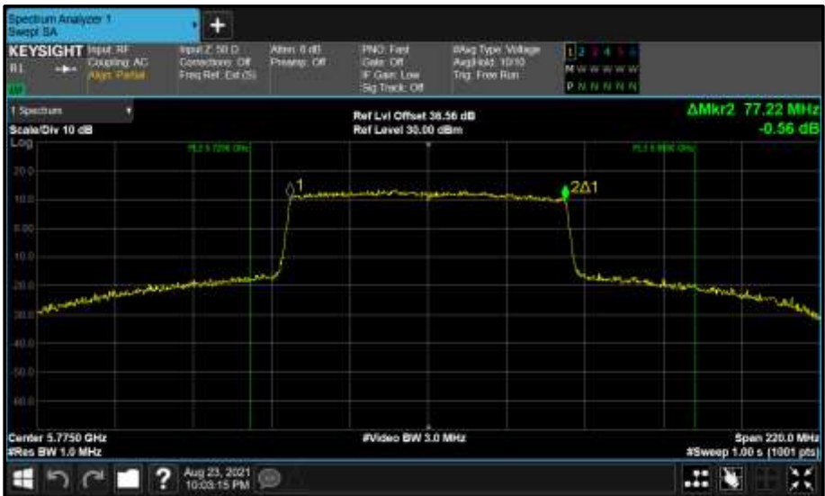
Figure 887 - Core 0 (A) 5775 MHz (CH155) 99% Bandwidth
