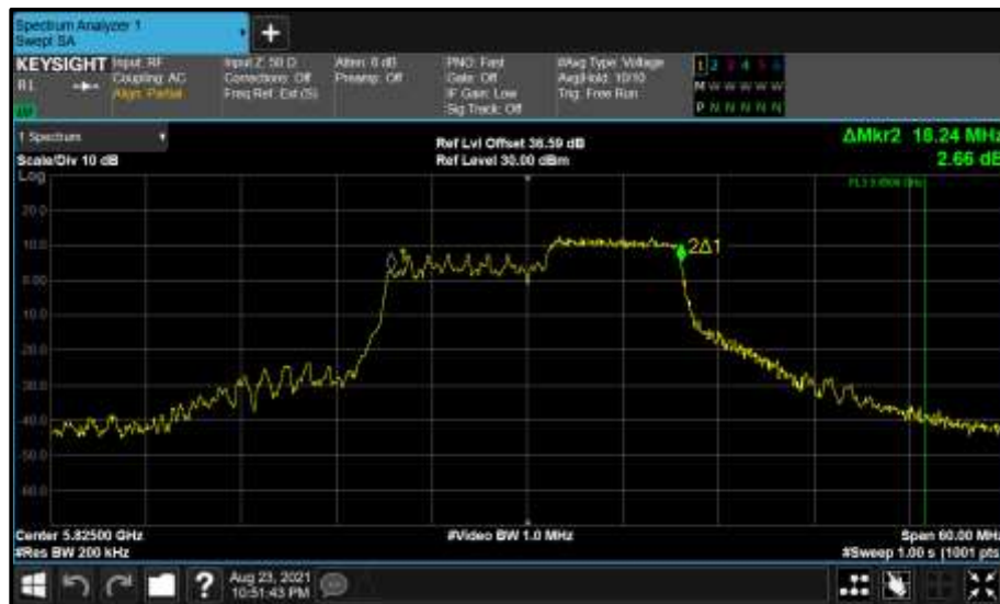
Figure 847 - Core 1 (B) 5825 MHz (CH165) 99% Bandwidth
