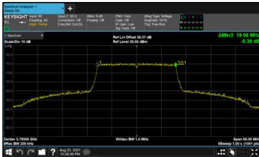
Figure 731 - Core 0 (A) 5785 MHz (CH157) 99% Bandwidth
