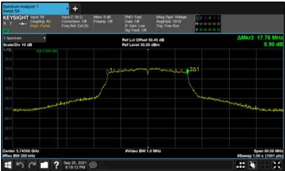
Figure 903 - Core 0 (A) 5745 MHz (CH149) 99% Bandwidth
