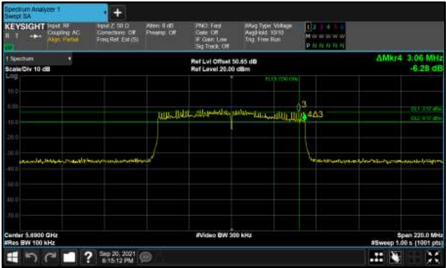
Figure 930 - Core 1 (B) 5690 MHz (CH138) 6 dB Bandwidth
