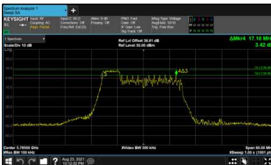
Figure 788 - Core 1 (B) 5785 MHz (CH157) 6 dB Bandwidth
