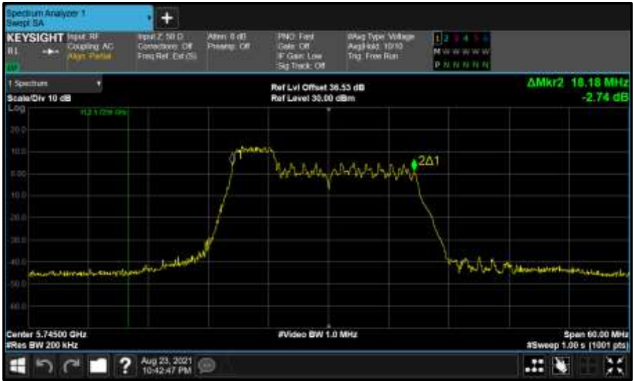
Figure 797 - Core 0 (A) 5745 MHz (CH149) 99% Bandwidth
