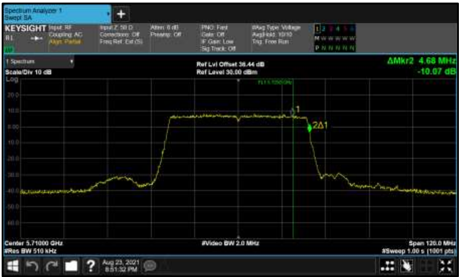
Figure 855 - Core 0 (A) 5710 MHz (CH142) 99% Bandwidth
