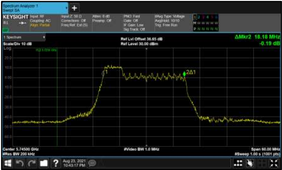
Figure 799 - Core 1 (B) 5745 MHz (CH149) 99% Bandwidth
