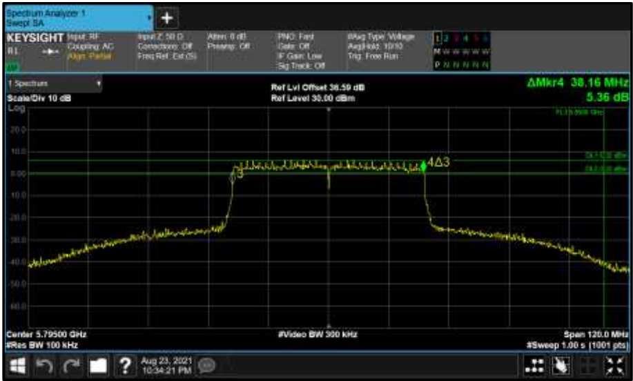
Figure 876 - Core 0 (A) 5795 MHz (CH159) 6 dB Bandwidth
