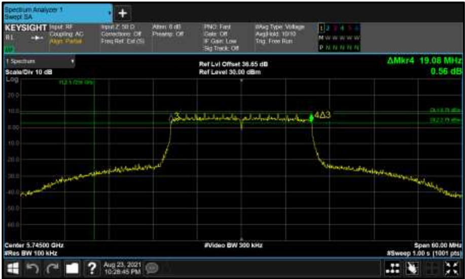
Figure 730 - Core 1 (B) 5745 MHz (CH149) 6 dB Bandwidth
