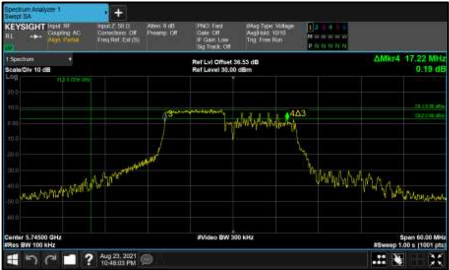
Figure 838 - Core 0 (A) 5745 MHz (CH149) 6 dB Bandwidth
