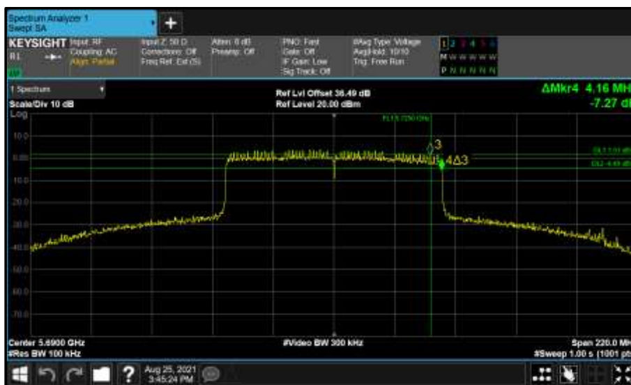
Figure 880 - Core 1 (B) 5690 MHz (CH138) 6 dB Bandwidth
