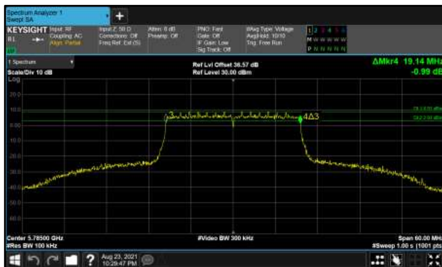
Figure 732 - Core 0 (A) 5785 MHz (CH157) 6 dB Bandwidth
