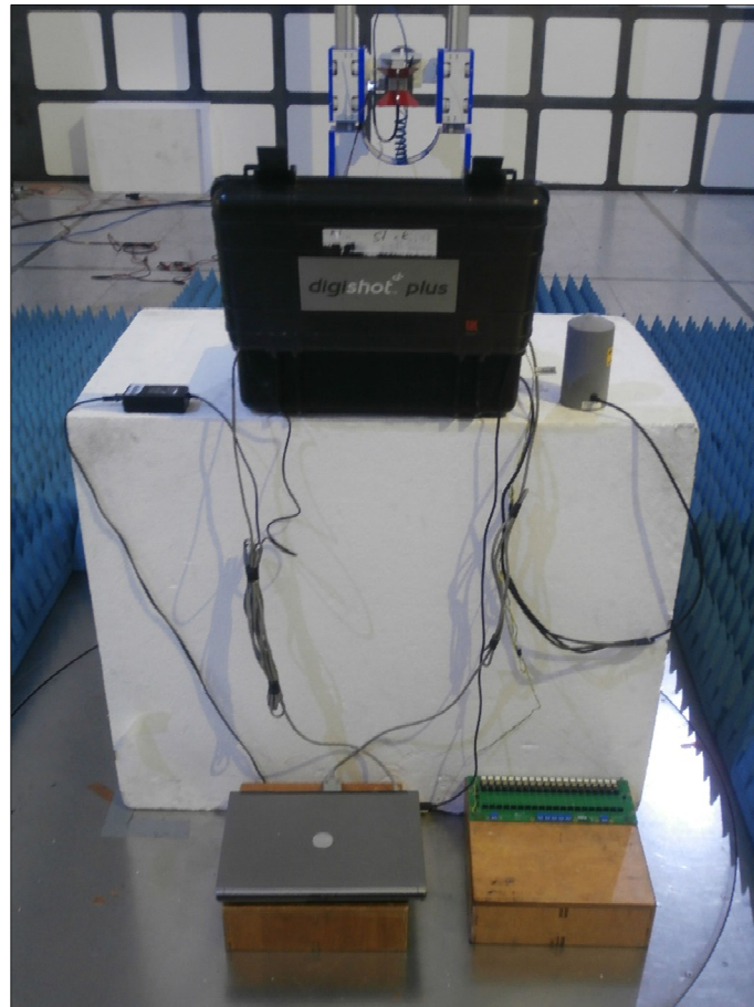
Figure 3 – Radiated Disturbance - 1 GHz to 5 GHz (FCC Part 15B, ICES-003 and RSS-GEN)
