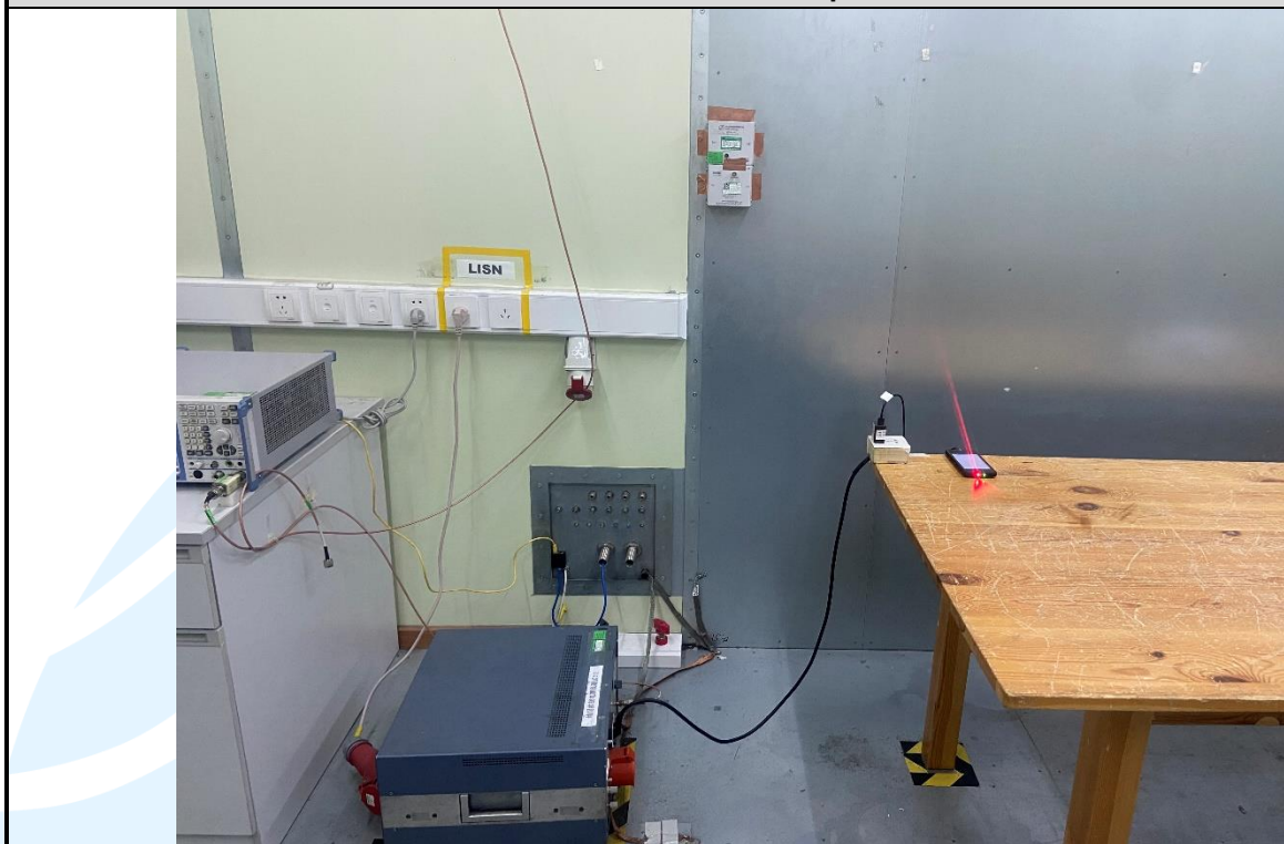
Conducted Emission Test Setup-3 – Test Mode 4
