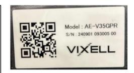
Description of how the labeling: Permanent adhesive labeling Explanation of the durability of the display:No peeling during expected lifetime FCC ID is displayed in a font size 4point or higher.
