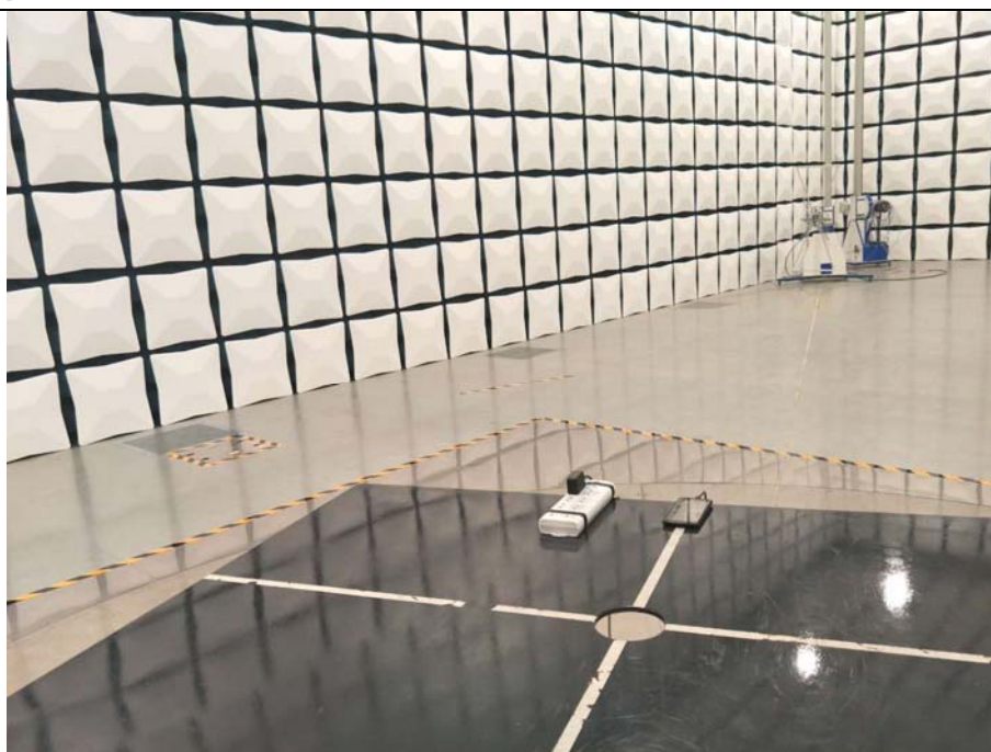
Spurious Radiated Emissions Test setup (below 1GHz)
