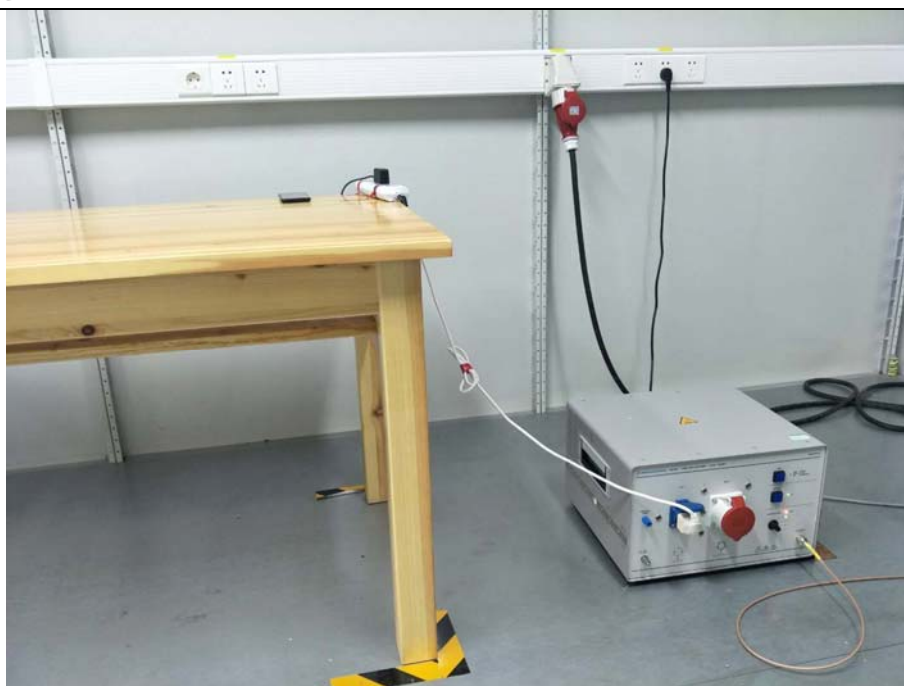
Conducted Emissions Test Setup (with charger)
