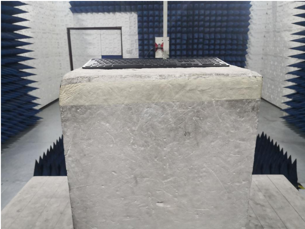
RADIATED EMISSION TEST SETUP ABOVE 1GHZ
