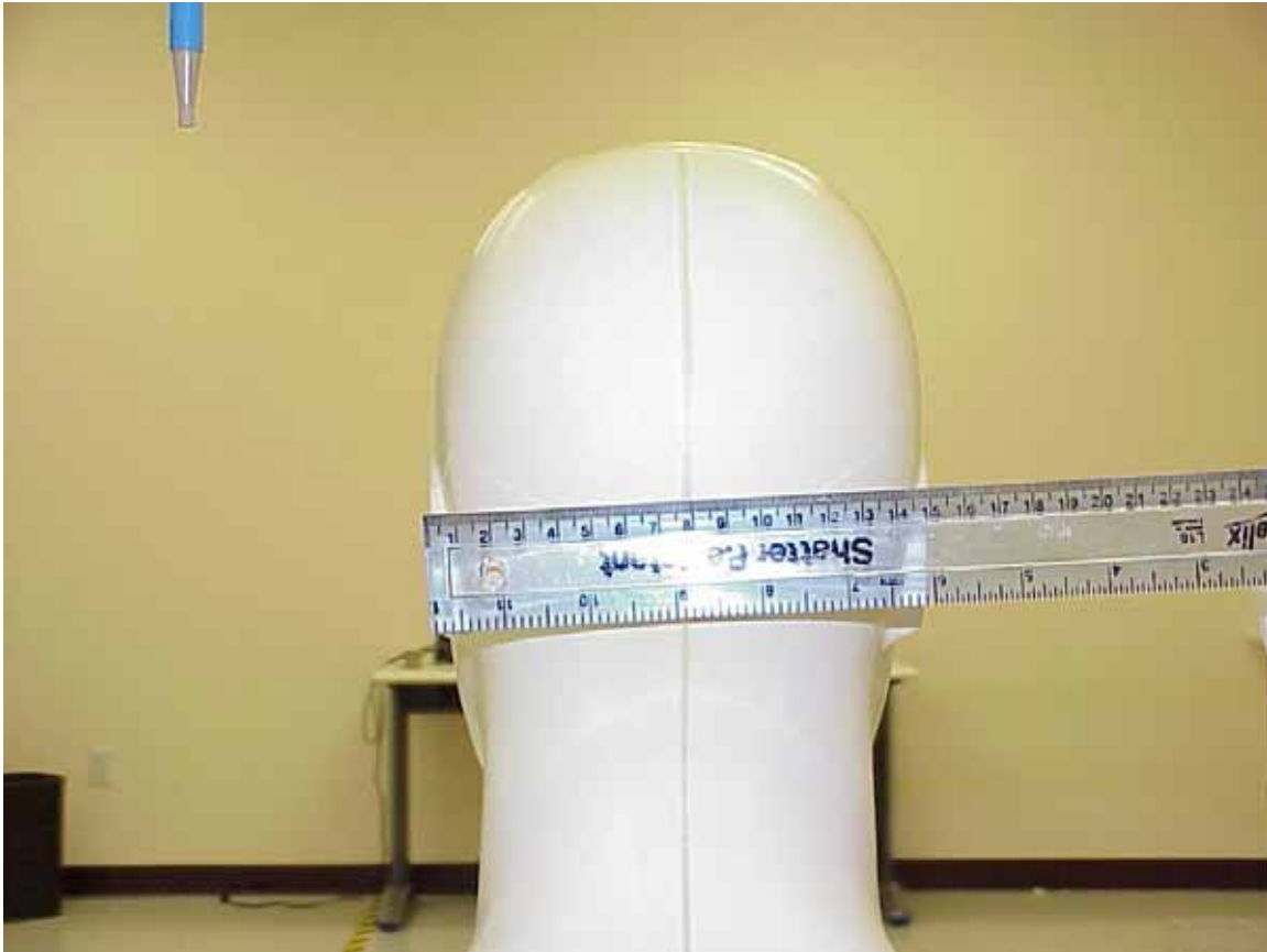
Photo 8. Photo to demonstrate 15 cm Z-axis head phantom
