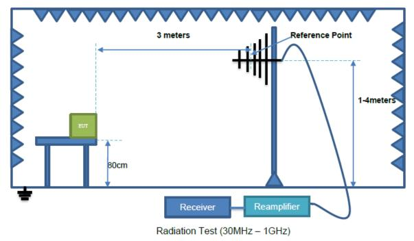
6.2 Test Standard and Limit FCC Part 15 Subpart C
