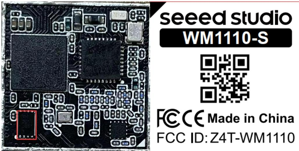
WM1110 has two models , the only difference between this two models is WM1110-S with encryption chip and WM1110-A not.
