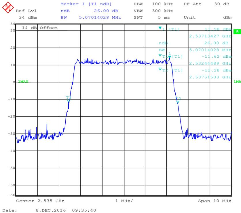
**QPSK (10 MHz) - 99% Occupied Bandwidth, Middle channel**
