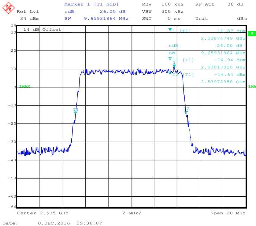
**QPSK (15 MHz) - 99% Occupied Bandwidth, Middle channel**
