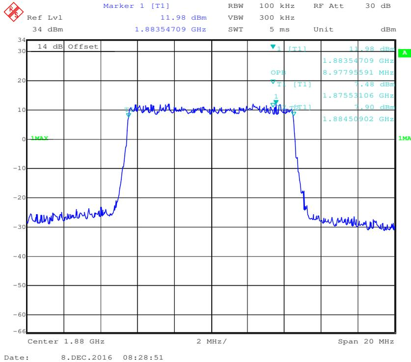
**QPSK (10.0 MHz) - 26 dB Bandwidth, Middle channel**
