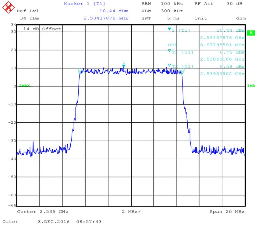
**16-QAM (10MHz) - 26 dB Bandwidth, Middle channel**
