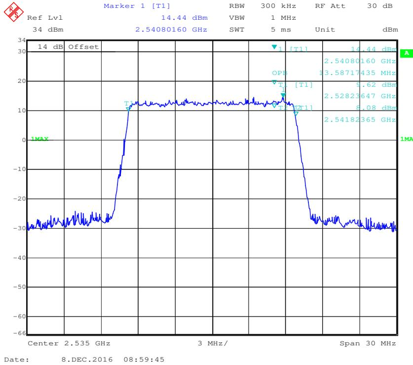
**16-QAM (15 MHz) - 26 dB Bandwidth, Middle channel**
