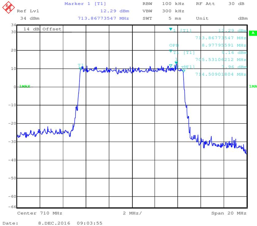
**16-QAM (10.0 MHz) - 26 dB Bandwidth, Middle channel**
