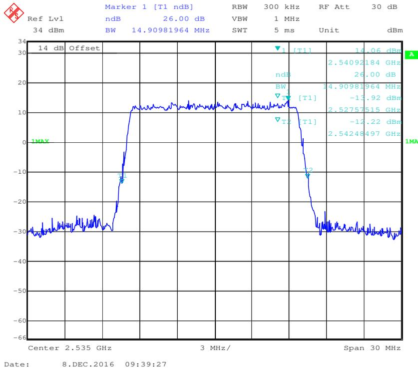
**16-QAM (15 MHz) - 99% Occupied Bandwidth, Middle channel**
