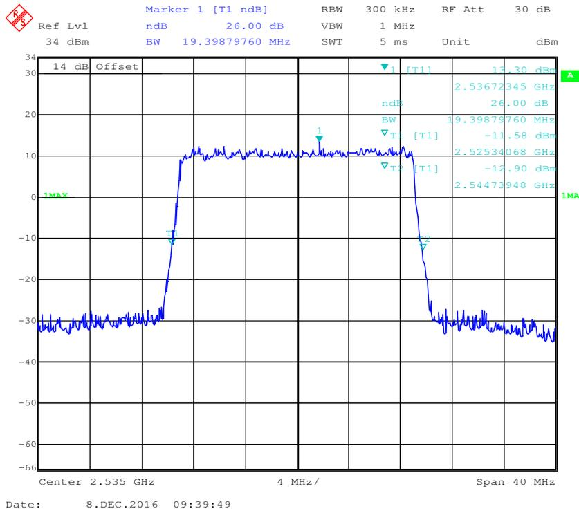
**16-QAM (20 MHz) - 99% Occupied Bandwidth, Middle channel**
