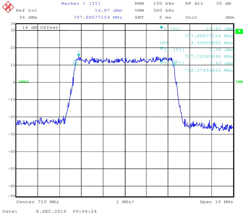
**16-QAM (5.0 MHz) - 26 dB Bandwidth, Middle channel**
