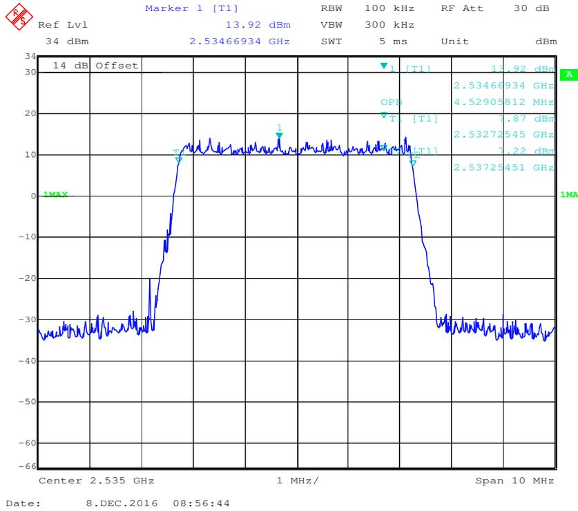
**QPSK (5 MHz) - 26 dB Bandwidth, Middle channel**
