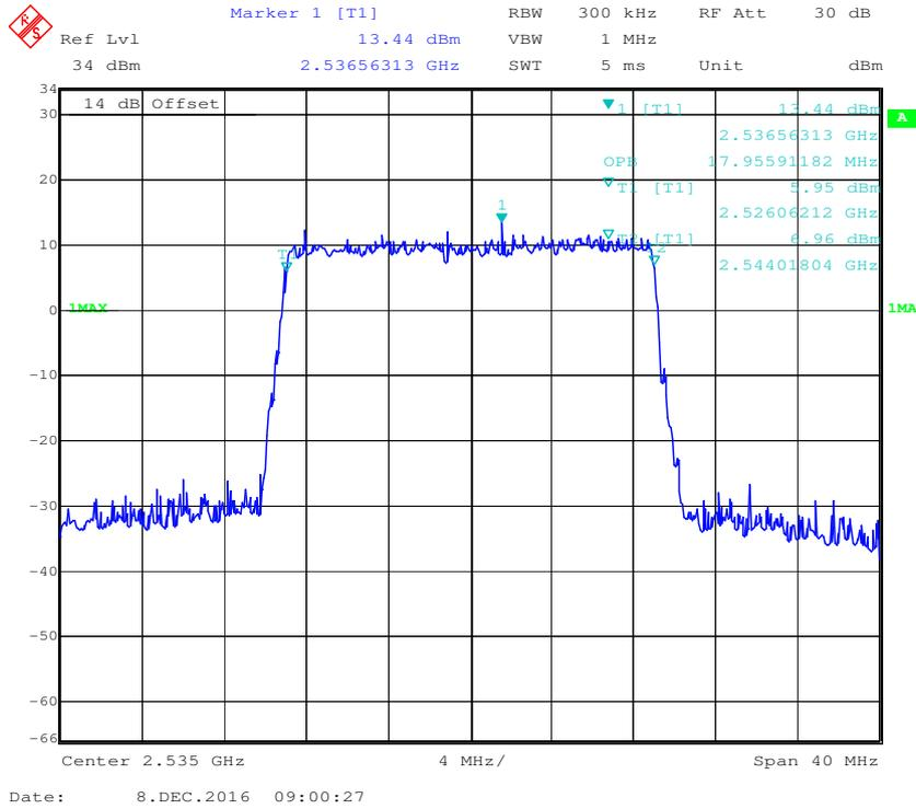
**QPSK (20 MHz) - 26 dB Bandwidth, Middle channel**
