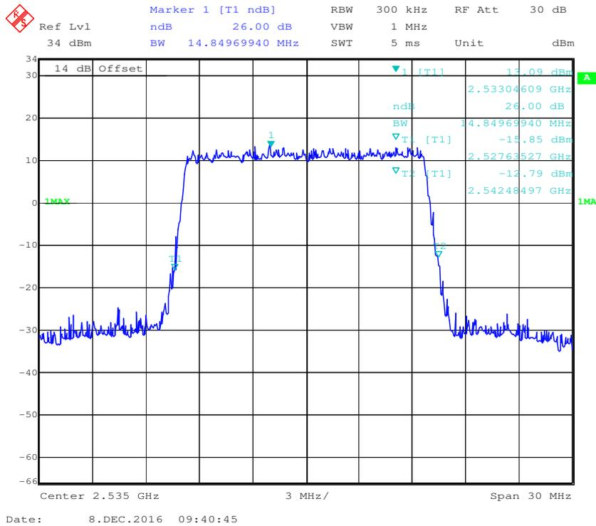
**QPSK (20 MHz) - 99% Occupied Bandwidth, Middle channel**
