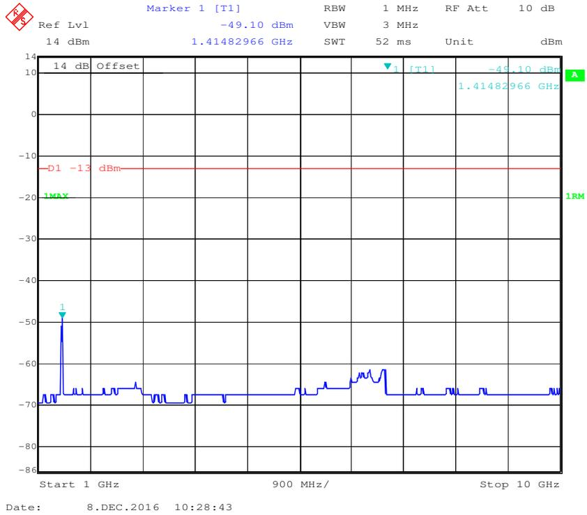
**FCC § 2.1053; § 22.917 (a); § 24.238 (a); § 27.53 (h)(m) SPURIOUS RADIATED EMISSIONS**
