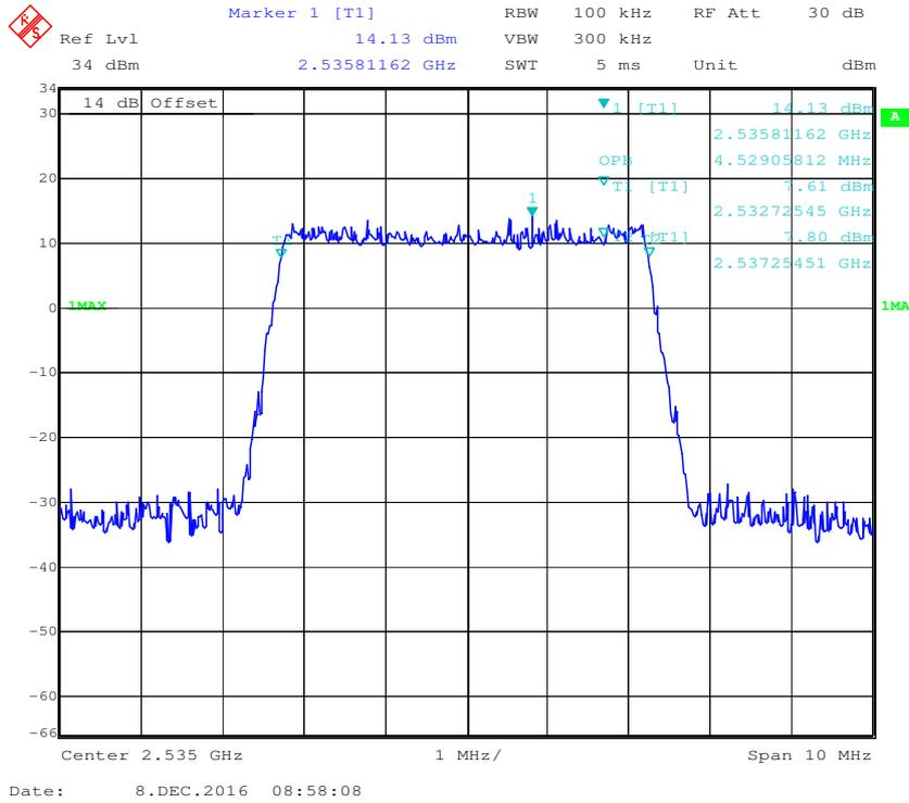
**16-QAM (5MHz) - 26 dB Bandwidth, Middle channel**
