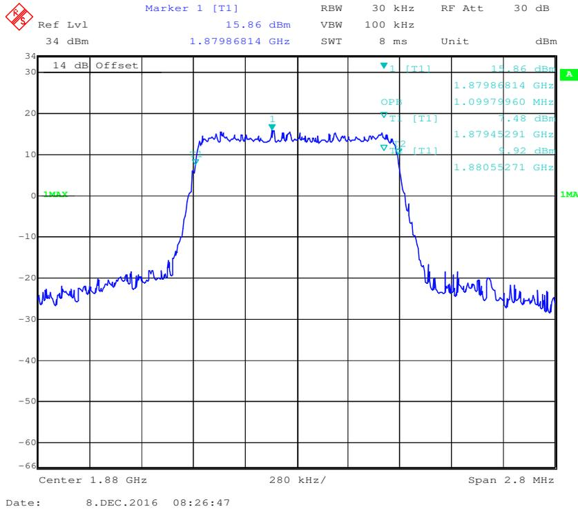
**16-QAM (1.4 MHz) - 26 dB Bandwidth, Middle channel**
