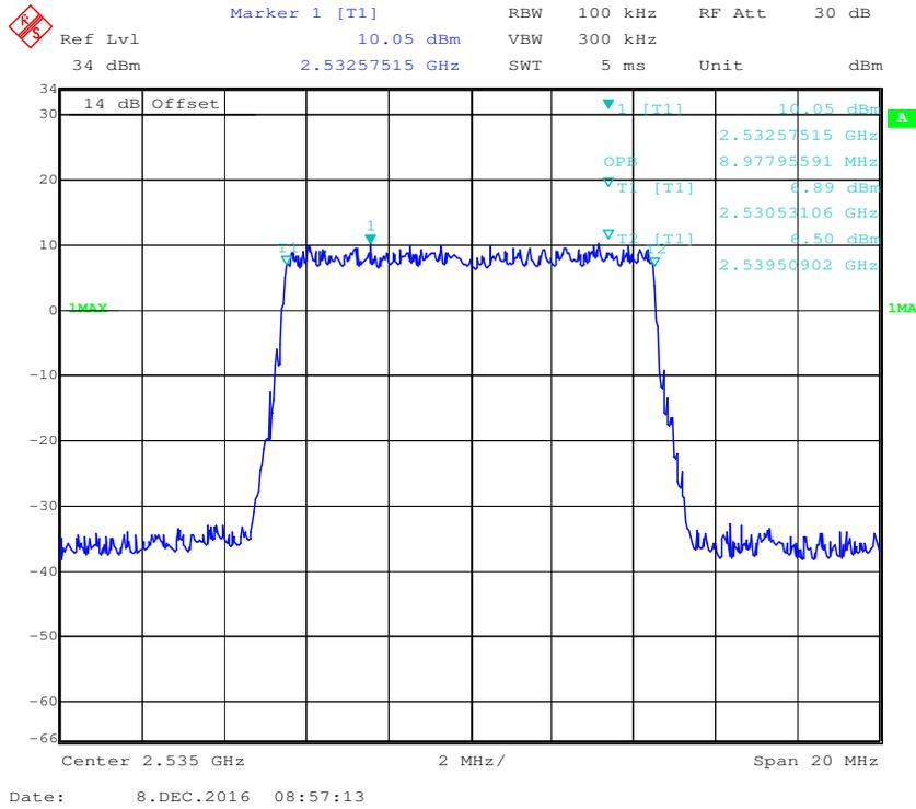
**QPSK (10 MHz) - 26 dB Bandwidth, Middle channel**
