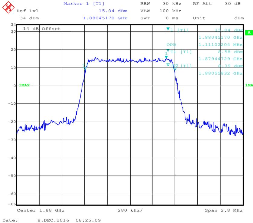
**QPSK (1.4 MHz) - 26 dB Bandwidth, Middle channel**
