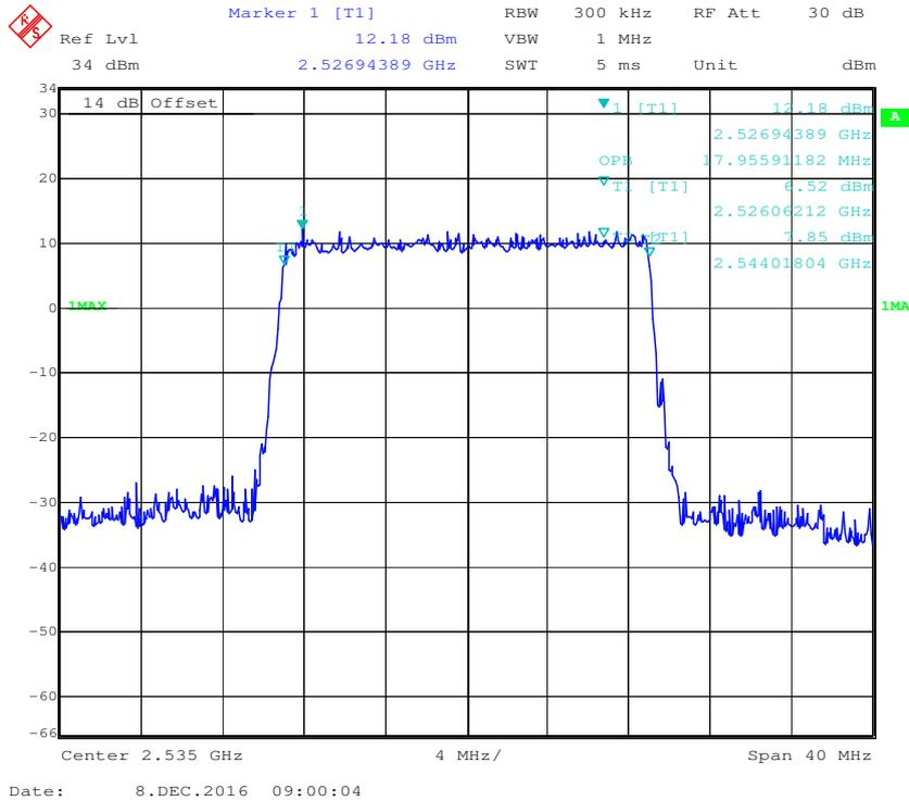
**16-QAM (20 MHz) - 26 dB Bandwidth, Middle channel**
