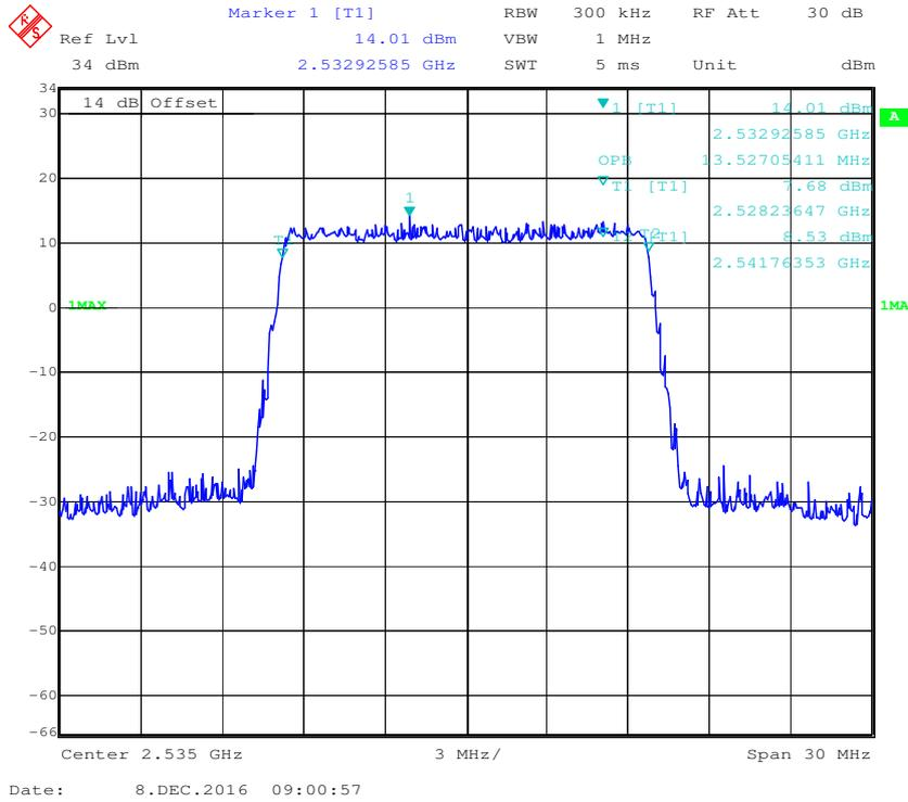
**QPSK (15 MHz) -26 dB Bandwidth, Middle channel**
