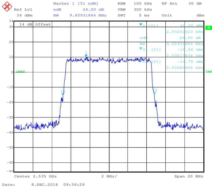
**16-QAM (10MHz) - 99% Occupied Bandwidth, Middle channel**
