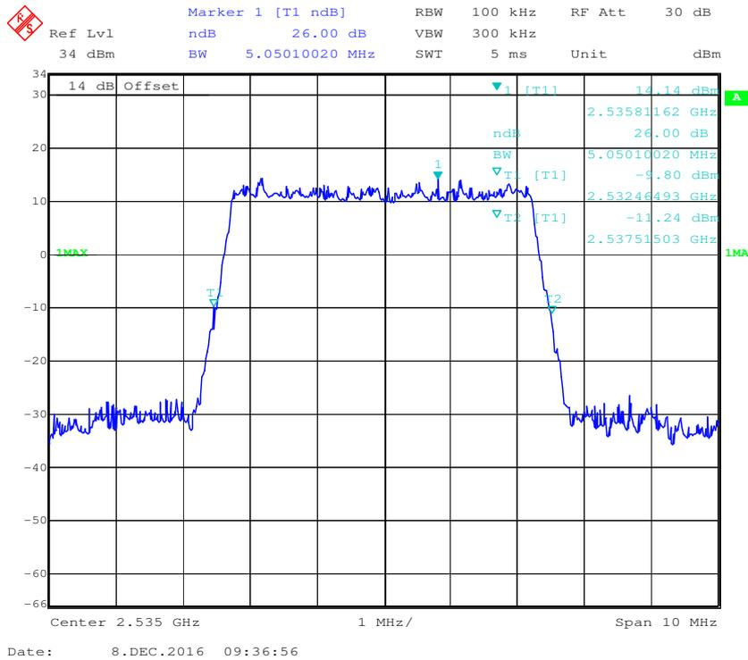
**16-QAM (5 MHz) - 99% Occupied Bandwidth, Middle channel**
