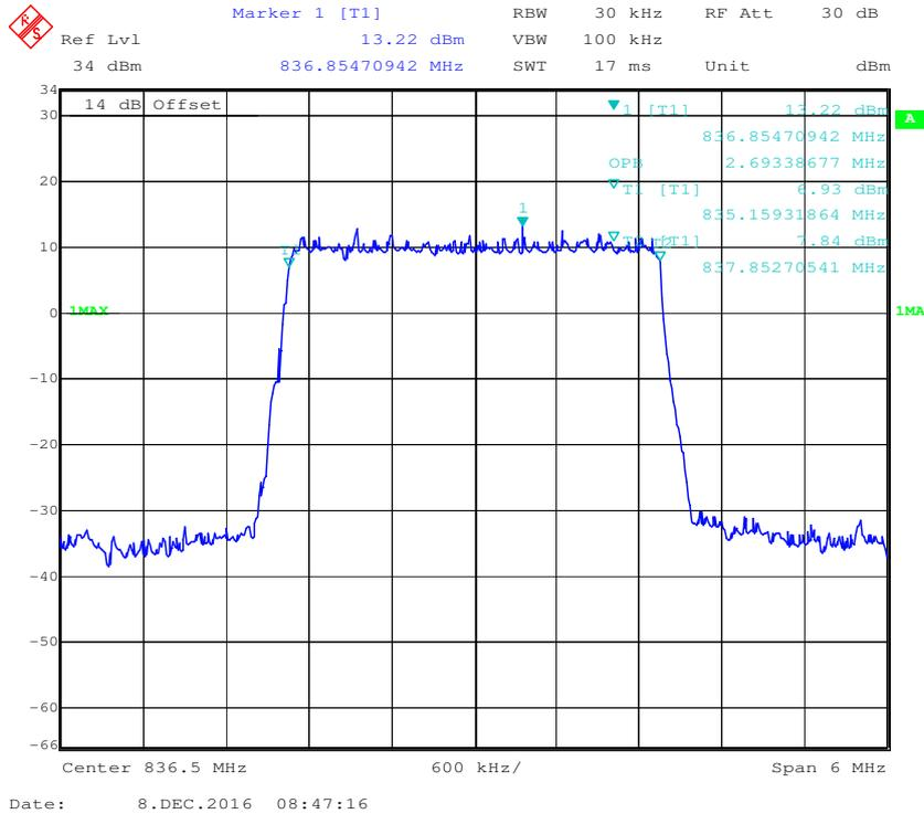
**16-QAM (3.0 MHz) - 26 dB Bandwidth, Middle channel**
