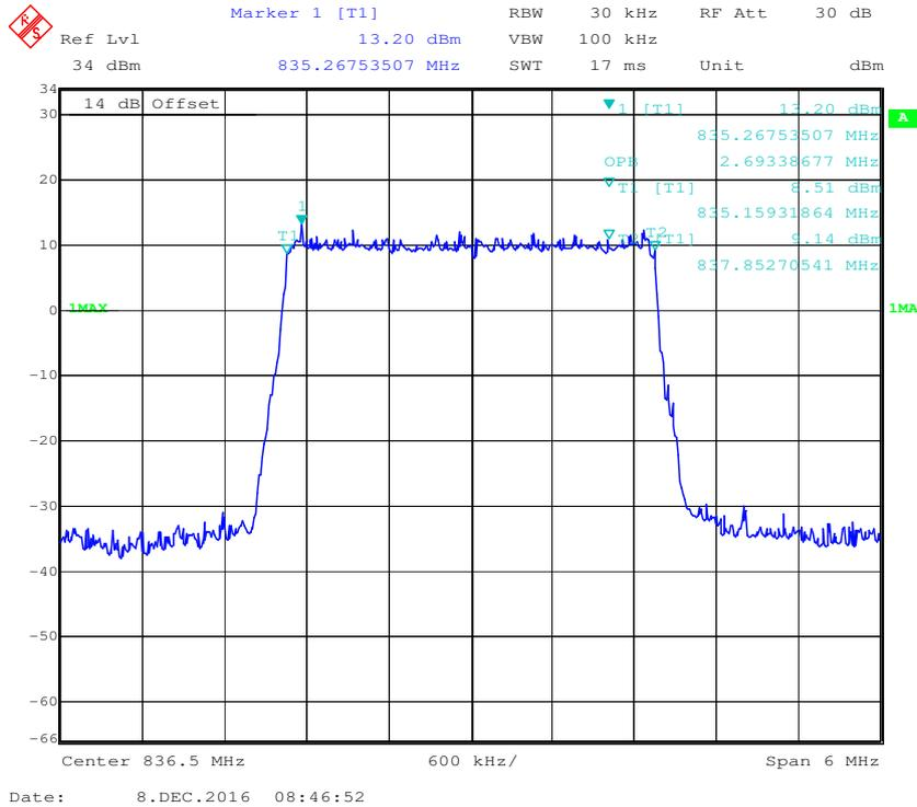
**QPSK (3.0 MHz) - 26 dB Bandwidth, Middle channel**
