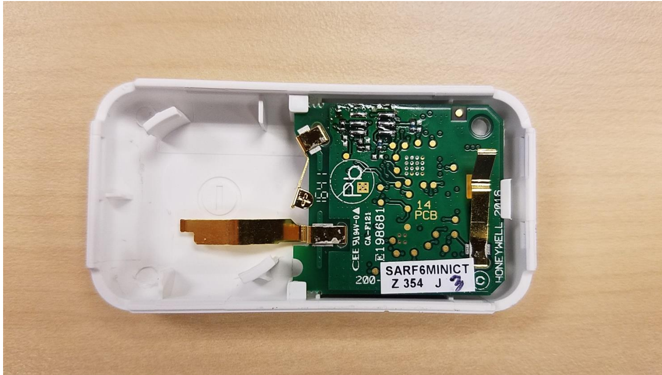
PCB Installed in Enclosure without Battery
