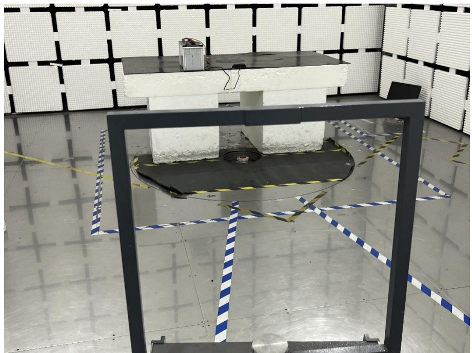
Radiation Emission Test Setup (Below 30MHz)
