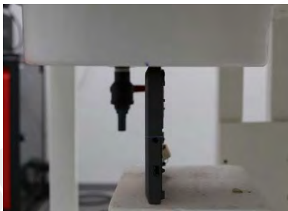
Fig.8 EUT Bottom side to flat phantom
