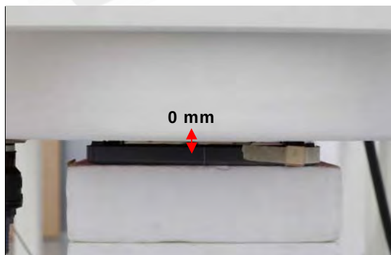
Fig.3 EUT Back side to flat phantom
