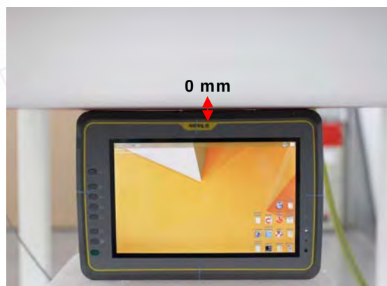
Fig.8 EUT Bottom side to flat phantom
