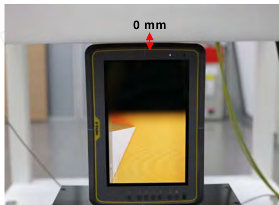
Fig.6 EUT Left side to flat phantom
