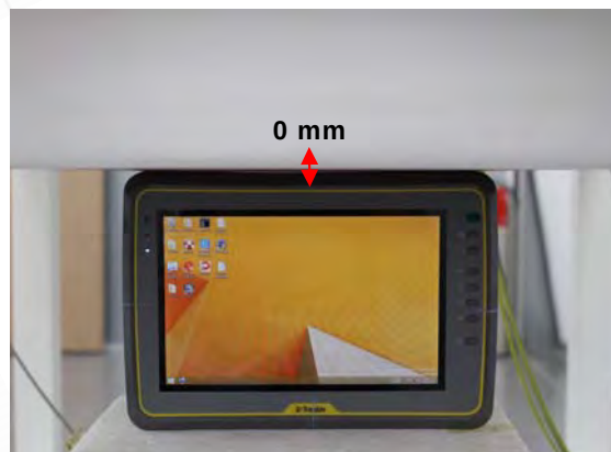
Fig.4 EUT Top side to flat phantom
