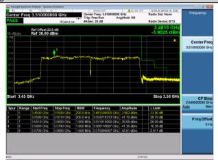
5G NR (3450-3550MHz) \_ SCS 30K Intra-band Continuous CA, Nominal Bandwidth: 20M+20M+20M \_ Low channel+ High channel
