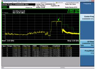
5G NR (3450-3550MHz) \_ SCS 30K Intra-band Continuous CA, Nominal Bandwidth: 40M+40M \_ Low channel+ High channel
