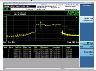
5G NR (3450-3550MHz) \_ SCS 30K Intra-band Continuous CA, Nominal Bandwidth: 10M+10M+10M+10M+10M+10M \_ Low channel+ High channel
