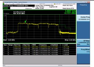
5G NR (3450-3550MHz) \_ SCS 30K Intra-band Continuous CA, Nominal Bandwidth: 10M+10M+10M+10M+10M \_ Low channel+ High channel
