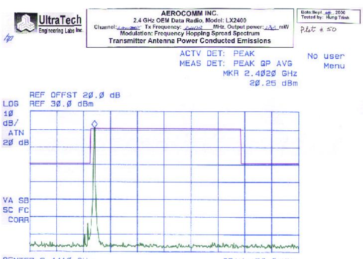
CENTER 2.441Ø GHz SPAN 150.0 MHz #IF BW 100 KHz #AVG BW 100 KHz SWP 45.0 msec
