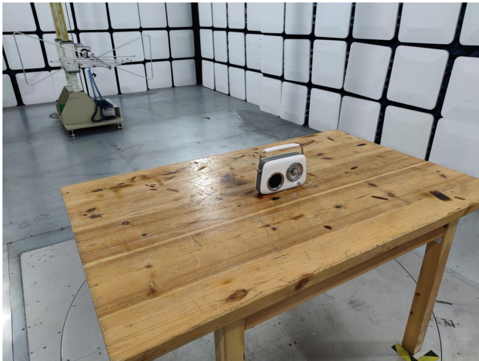
Photo of Radiation Emission Test
