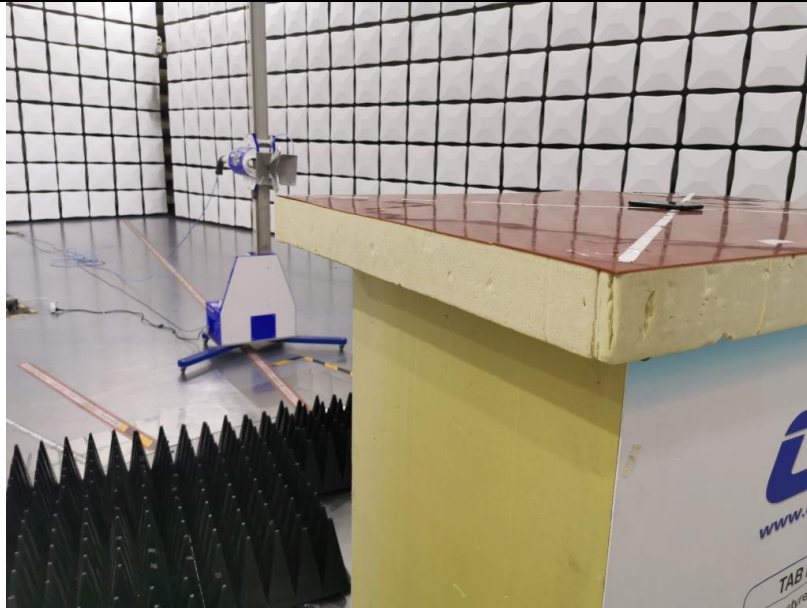
Spurious Radiated Emissions Test setup
