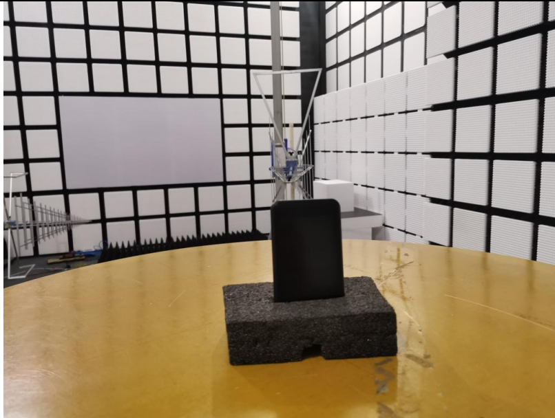
Spurious Radiated Emissions Test setup
