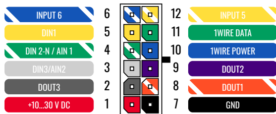
FMC13A 2x6 socket pinout
