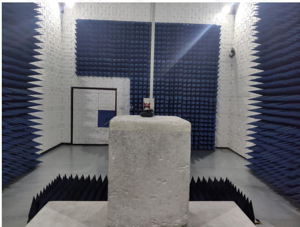
FCC RADIATED EMISSION TEST SETUP ABOVE 1GHZ
