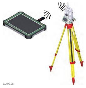
Standard setup at the CS35 for remote surveying using the CTR35.
