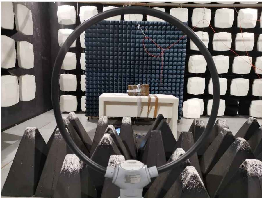
Photograph 12: EUT test setup 2 in the semi anechoic chamber, close up view_EUT elevation 90°, EUT in TXRX mode
