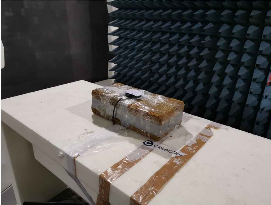
Photograph 9: EUT test setup 2 in the semi anechoic chamber, close up view_EUT elevation 0°, EUT in TXRX mode
