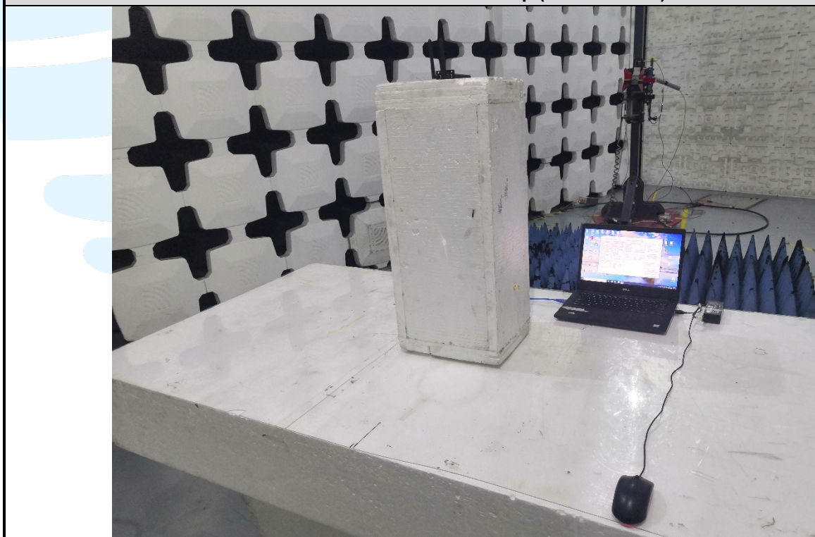
Radiated emission Test Setup (Above 1 GHz)
