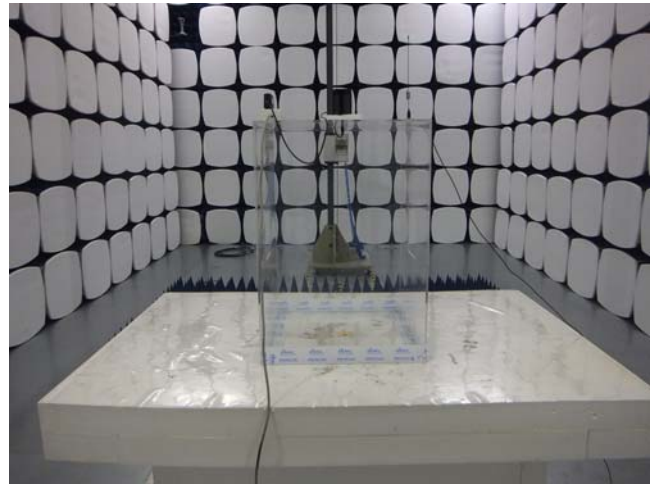
Radiated Spurious Emissions Test Setup Above 1GHz
