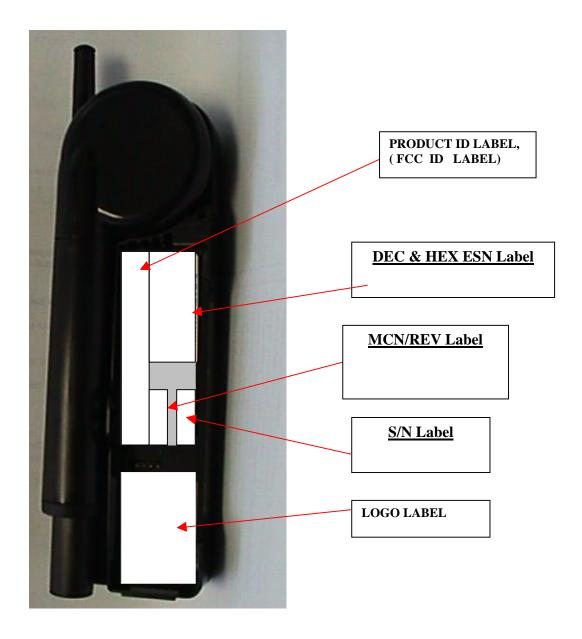
Labels are in same location, on back of phone beneath external battery, for both the Tri-mode Portable UT (shown above) and the Single-Mode Portable UT.
