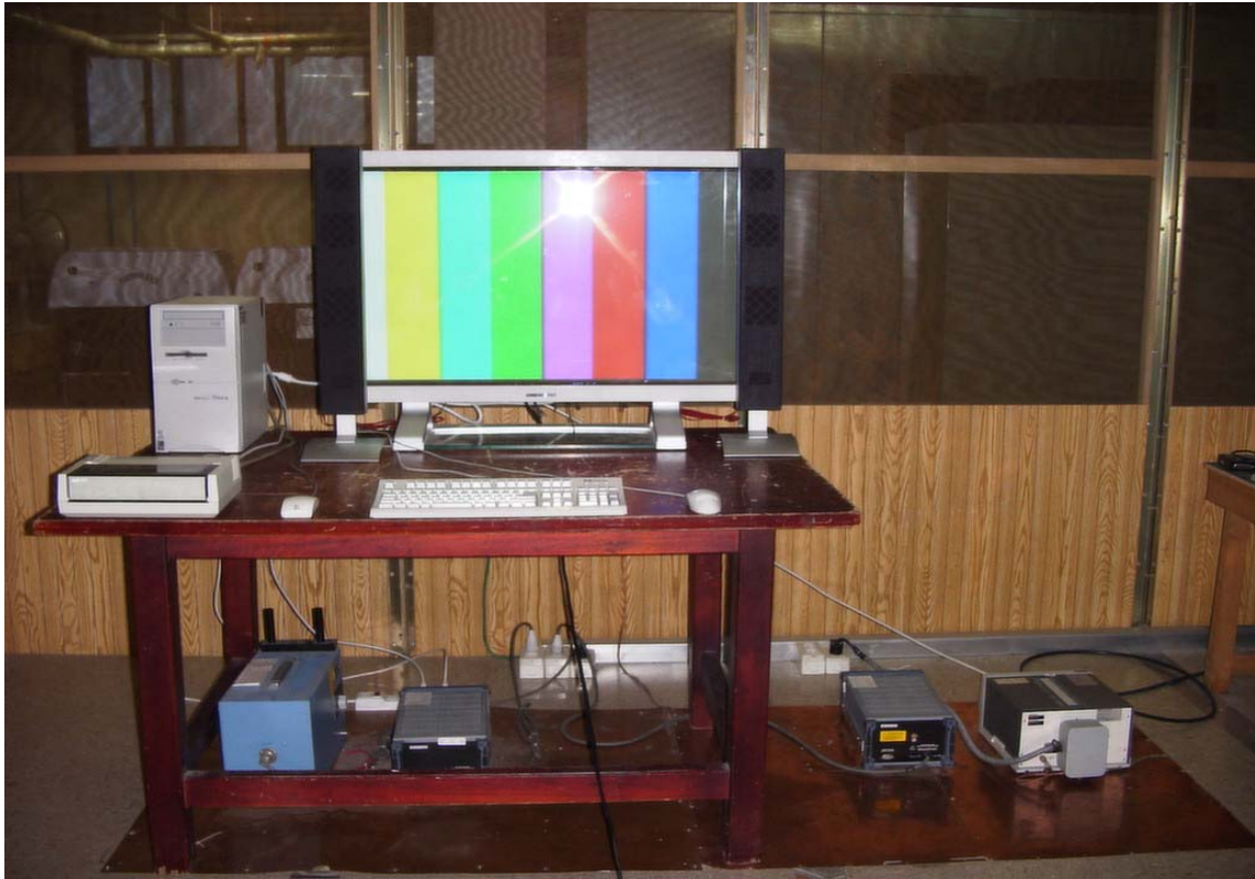
Conducted Emission 450kHz ~ 30MHz Mode : Color bar
