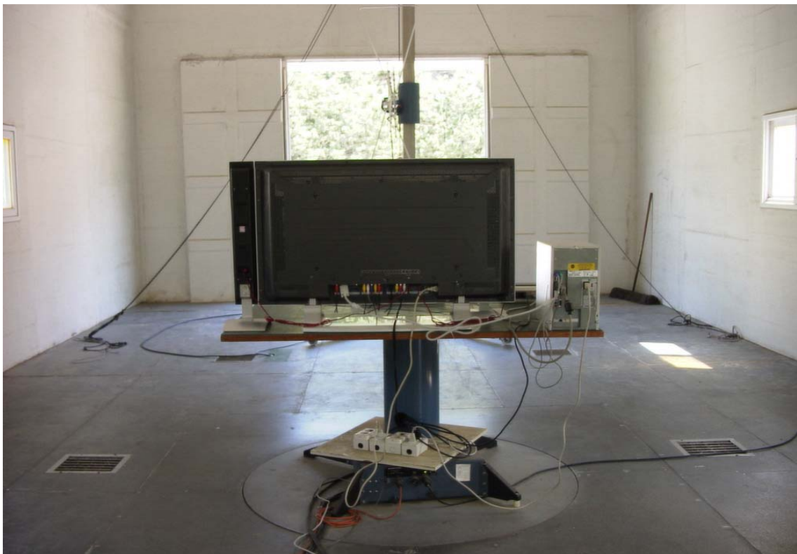
Radiated Emission 30MHz ~ 1000MHz Mode : Scrolling "H" Pattern
