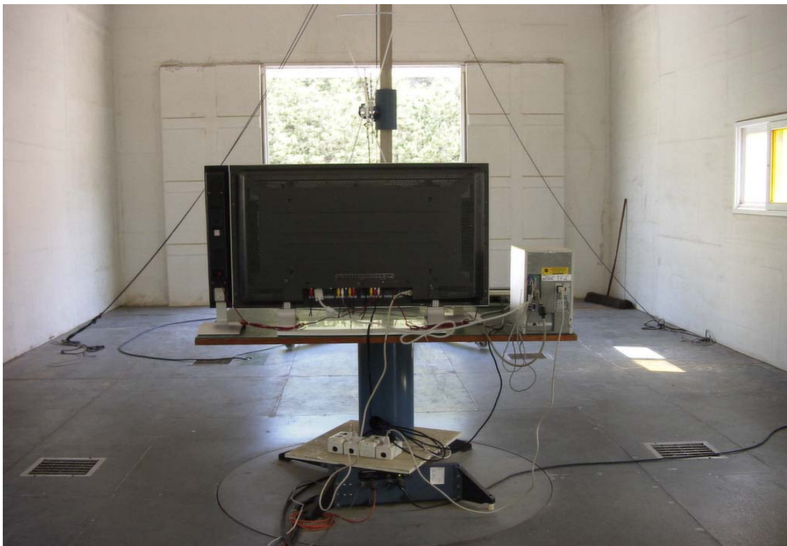
Radiated Emission 30MHz ~ 1000MHz Mode : Color bar
