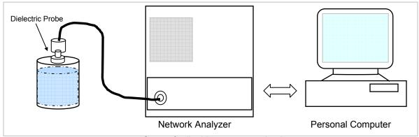
Set-up for liquid parameters check
