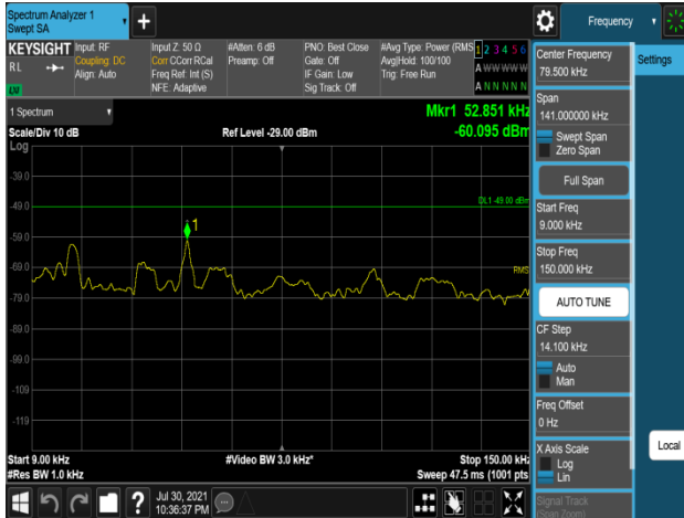
Plot 7-1003. Conducted Spurious Emission Plot 9 kHz to 150 kHz (B2_5M_1C_QPSK - Mid Channel, Port 1)
