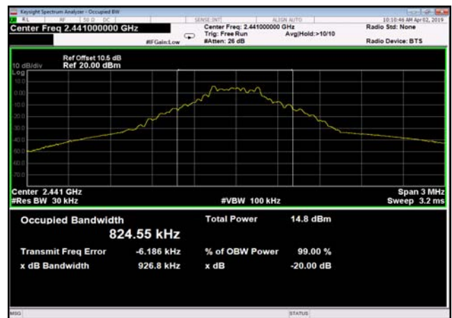
20dB Bandwidth: DQPSK,2402MHz,2DH5
