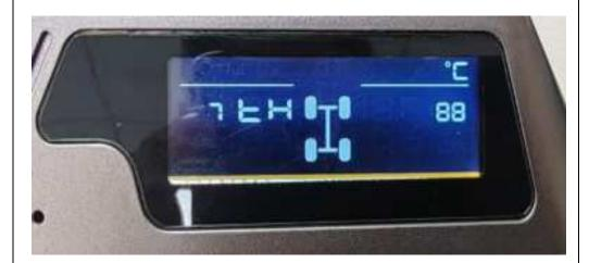
**8.** Pairing mode Long Push the middle button for 3 seconds to enter the settings menu. Short press the right button, "8" will be displayed in the top left corner.Pairing in this mode.
