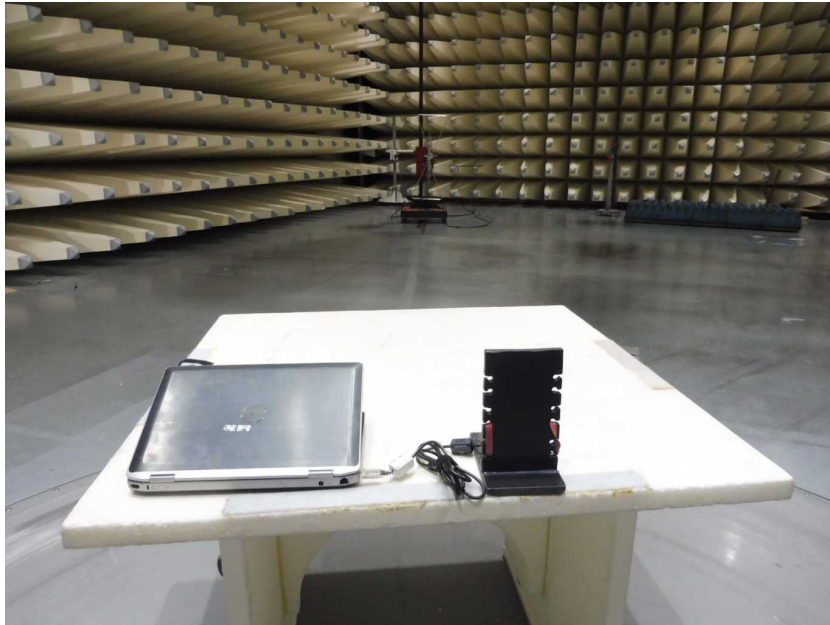
Photo 11: EUT at the semi-anechoic chamber
